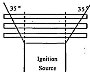
Figure 12: Cable tray stack fire propagation model
