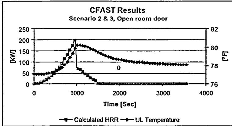
Figure 19: CFAST results for upper layer and heat release rate in scenario 2 & 3.
