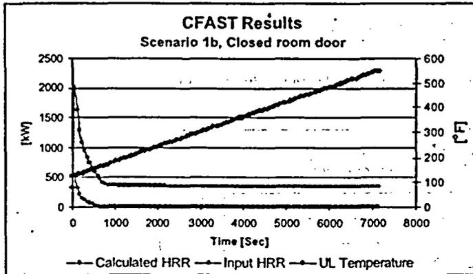
Figure 17: CFAST results for upper layer and heat release rate in scenario 1b.
