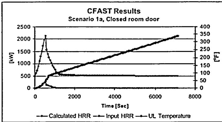
Figure 15: CFAST results for upper layer and heat release rate in scenario 1a.
