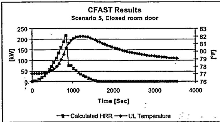
Figure 22: CFAST results for upper layer and heat release rate in scenario 5.
