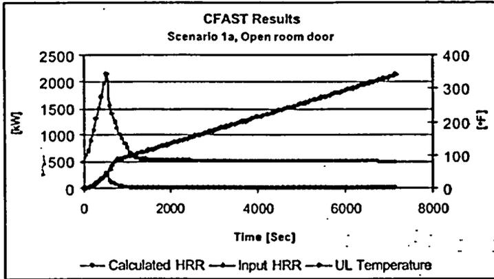
Figure 14: CFAST results for upper layer and heat release rate in scenario 1a.
