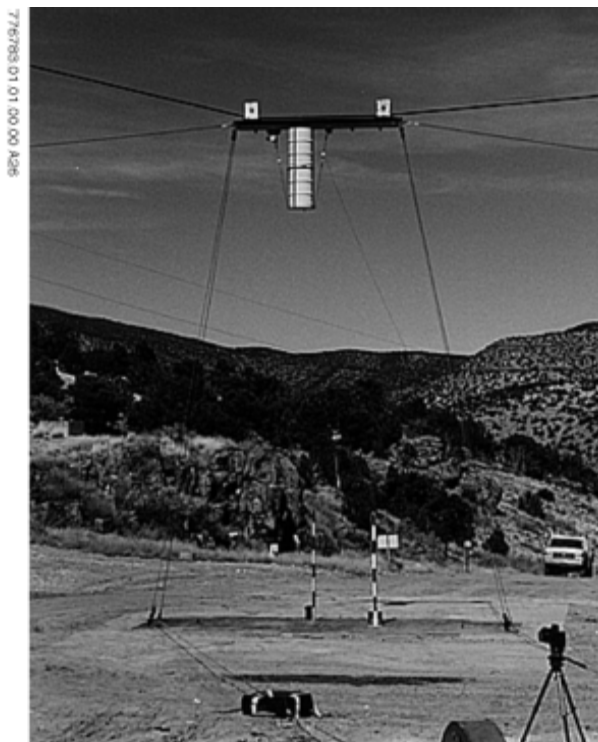
Figure 4.1-3b. Top-Impact Drop Test Set-up
