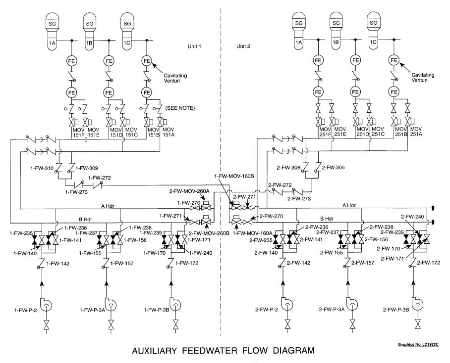
NOTE: Letter Serial No. 03-636, dated February 9, 2004, committed to install stop check valves downstream of each of the AFW Steam Generator Isolation MOVs. The valves have been installed on Unit 1 and will be installed on Unit 2 during the 2005 refueling outage.
