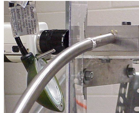
Camera and light focused on flaw
