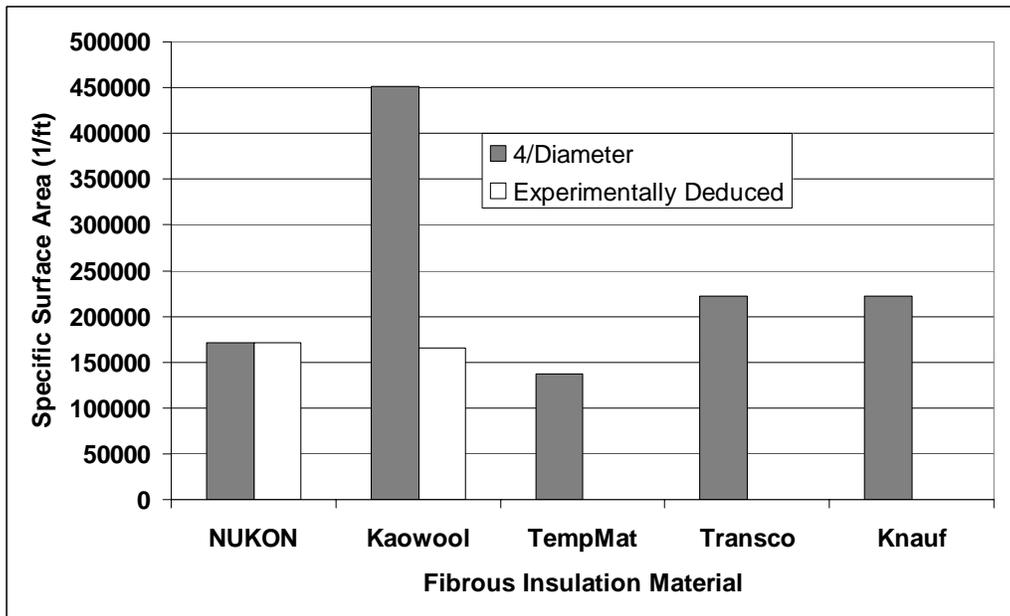
Figure V-4. Comparison of Fibrous Insulation Specific Surface Areas
