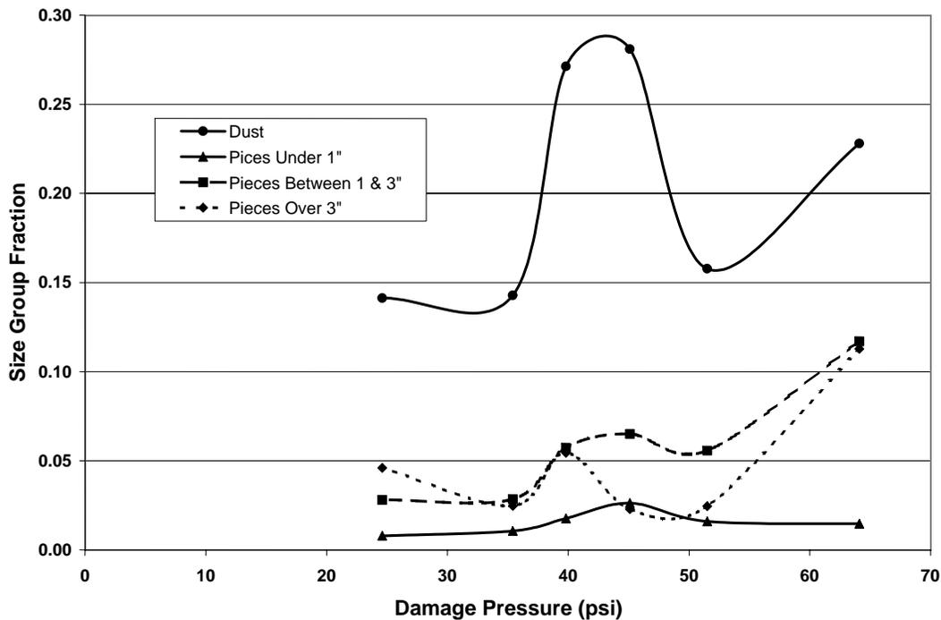
Figure VI-5. Debris-Size Distributions for OPG Calcium Silicate Tests
