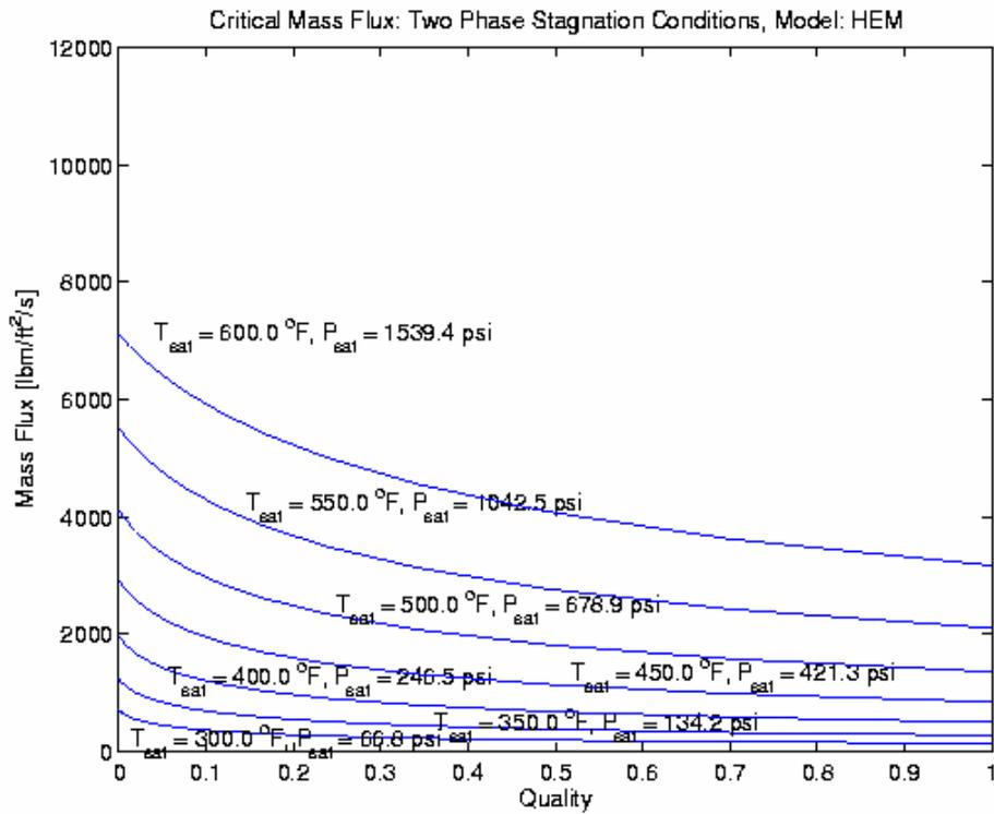
Figure I-7. HEM Critical Mass Flux, Saturated Stagnation
