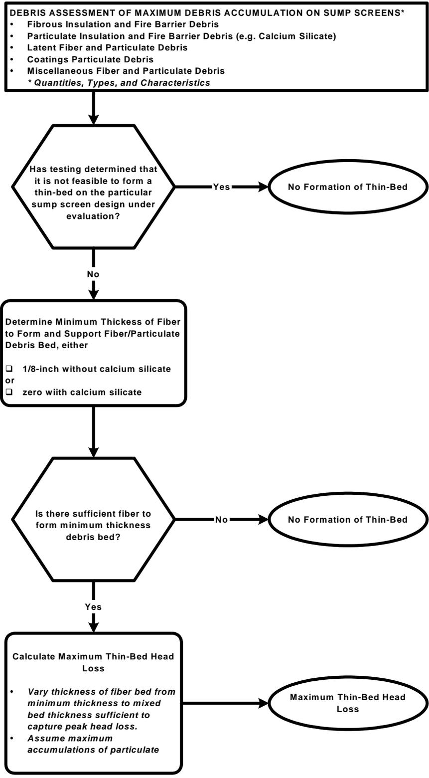
Figure VIII-11 Procedure for Estimating Conservative Thin-Bed Head Losses
