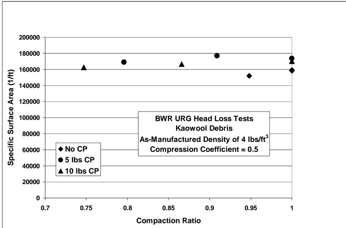
Figure V-3. Kaowool™ Specific Surface Area Using Modified Parameters
