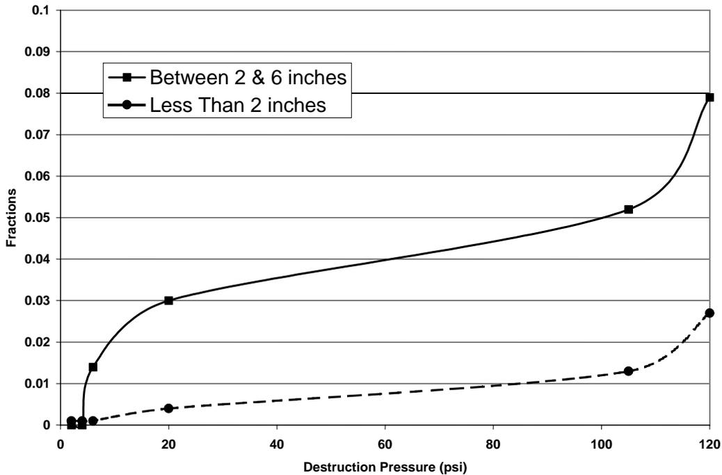
**Figure VI-4. Relative Damage of Stainless-Steel DPSC MIRROR™ Insulation**
