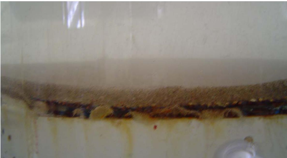
**Figure VIII-4. Debris Bed for the Surrogate Latent Particulate Head-Loss Test 16**
