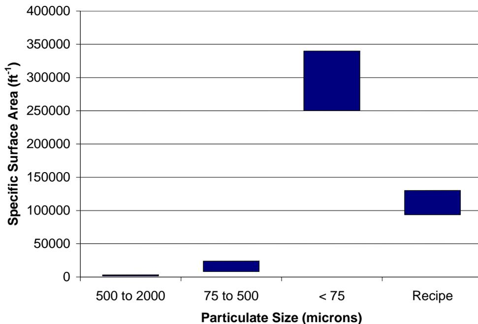
**Figure V-6. Comparison of Component and Recipe Specific-Surface-Area Ranges**
