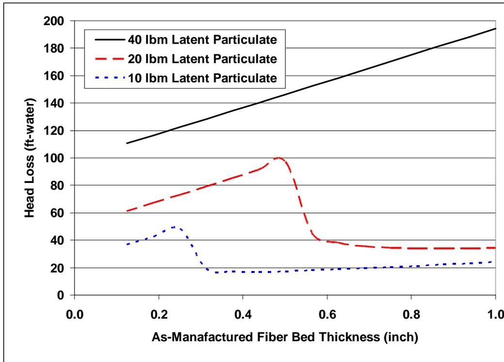
**Figure VIII-9. Parametric Example of Peak Head-Loss for Given Mass of Particulate**
