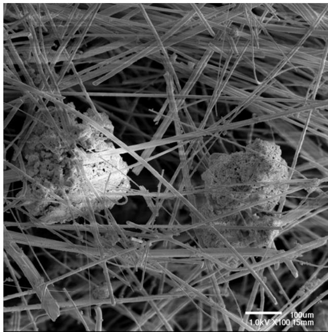
**Figure VIII-1. Example of Particulate Embedded in Fibrous Debris<sup>1</sup>**
