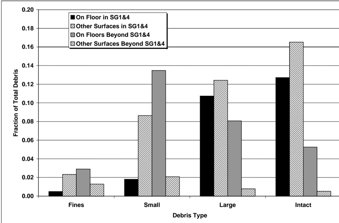
Figure VI-12. Blowdown Debris Dispersion by Surface Orientation
