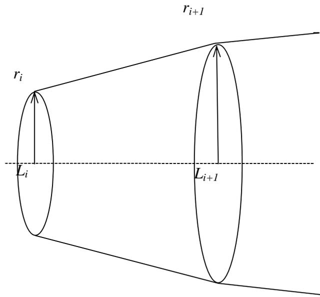
Figure I-3. Linear Segmentation of Jet Cross Sections for Numerical Volume Integration
