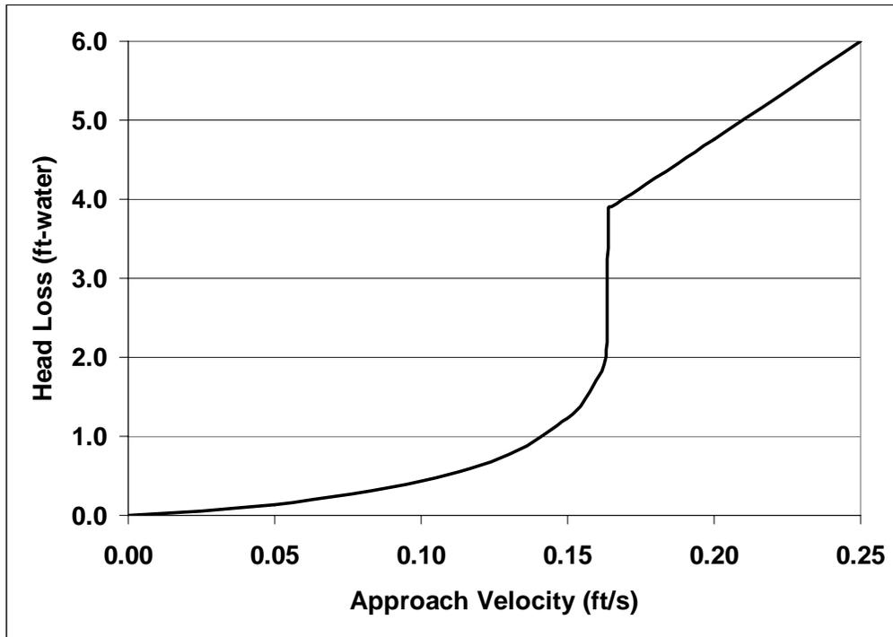
Figure VIII-6 Head Loss Example of Thin-Bed Formation Due to Bed Compression
