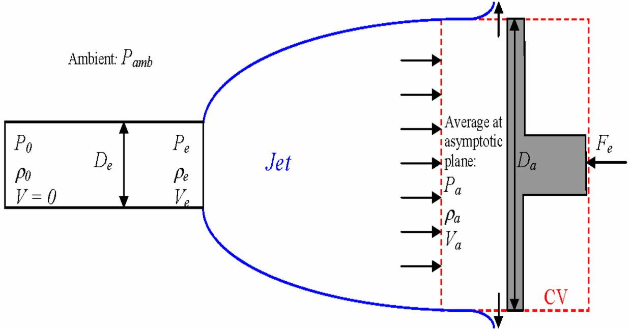
Figure I-4 through Figure I-7 show thrust coefficients computed using pressures and fluid properties evaluated from the HEM and Henry-Fauske models. Regardless of the model, the value of  $C_T$  approaches 2.0 for incompressible, highly subcooled liquid and approximately 1.26 for saturated steam. These results agree with theory and are recommended for use in the standard.
