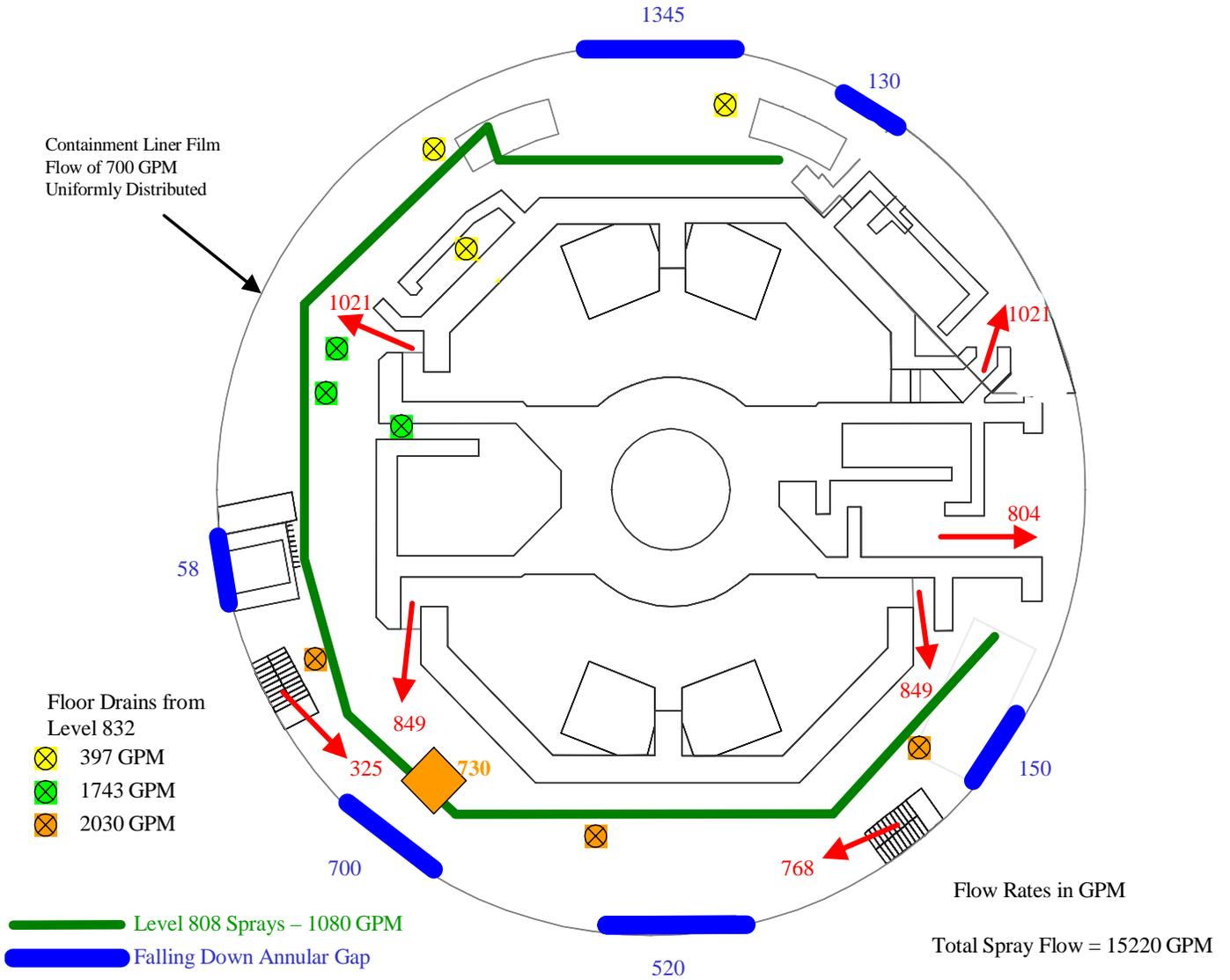
**Figure 7. Spray-Water Drainage to Level 808 Sump Pool**
