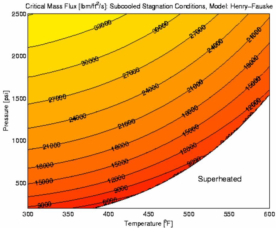
Figure I-6. Henry-Fauske Critical Mass Flux, Subcooled Stagnation
