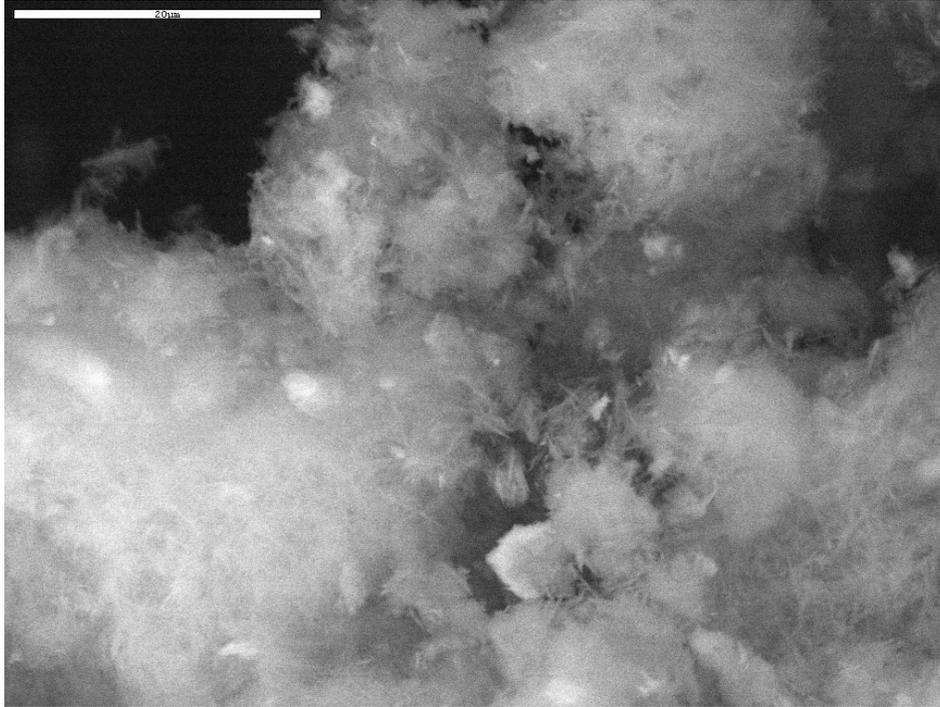
**Figure VIII-2. Pretest SEM Photo of Calcium Silicate Particulate Debris**
