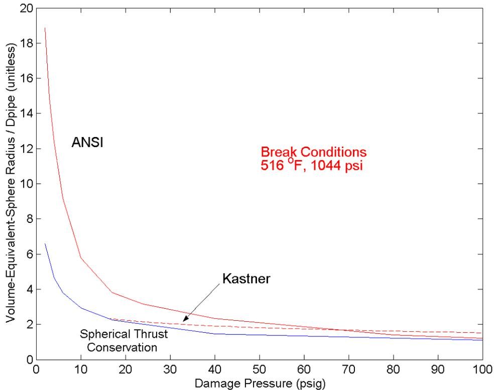
**Figure I-26.** Comparison of Equivalent Spherical Damage Radii
