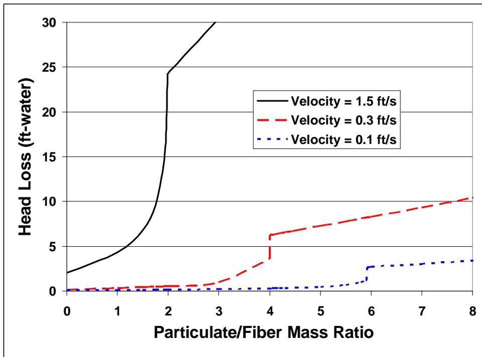
**Figure VIII-8. Parametric Example of Thin-Bed Formation**
