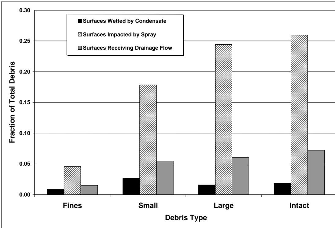
Figure VI-13. Blowdown Debris Dispersion by Surface Wetting
