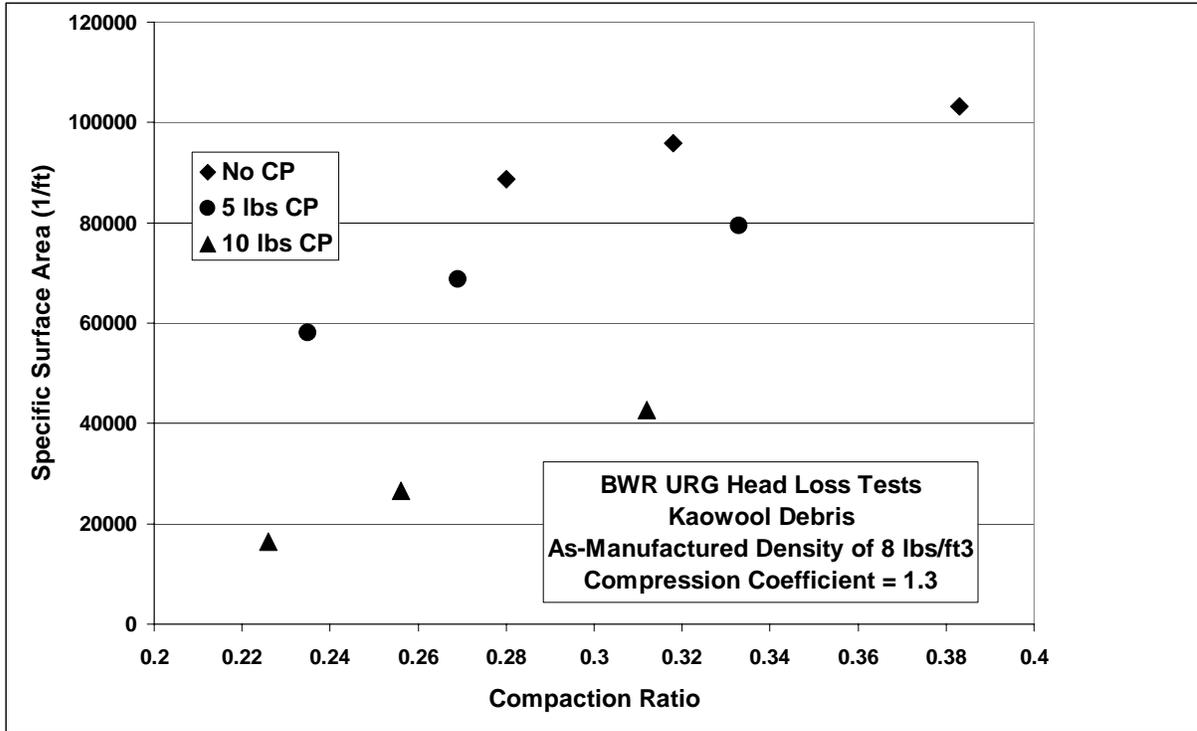
**Figure V-2. Kaowool Specific Surface Area Assuming Base Parameters**
