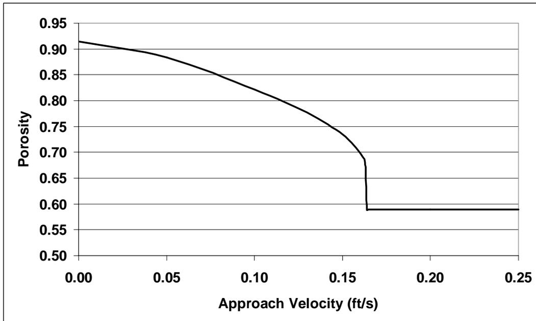
Figure VIII-7 Porosity Example of Thin Bed Formation Due to Bed Compression
