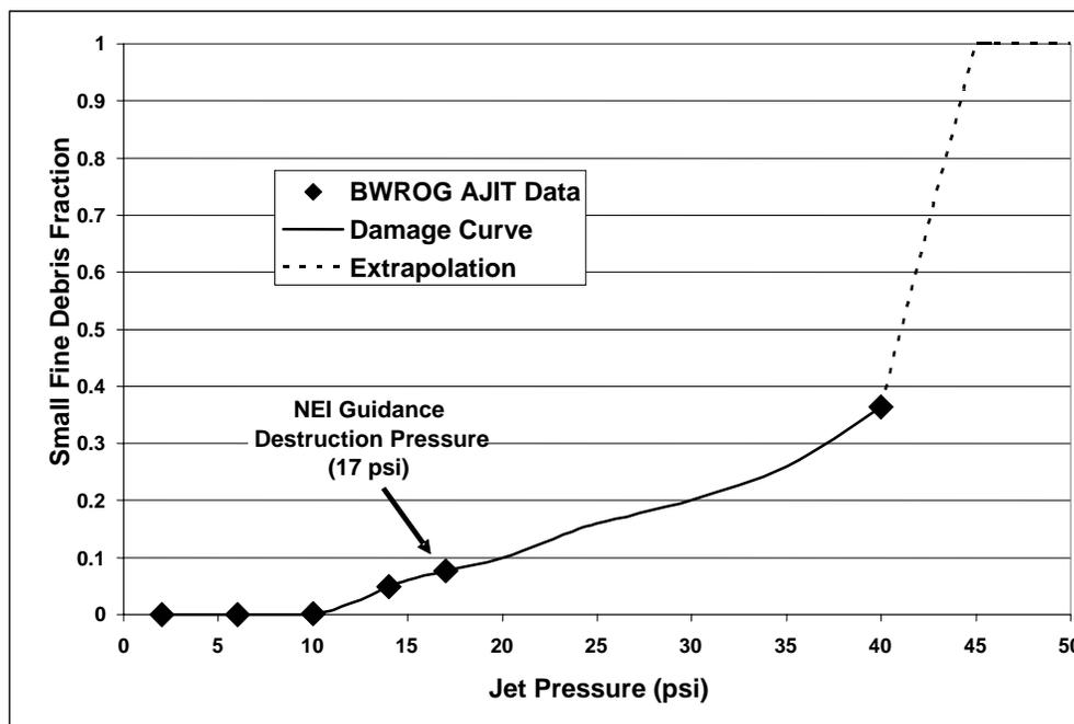
**Figure II-4. Temp-Mat Damage Curve for Small Fine Debris**
