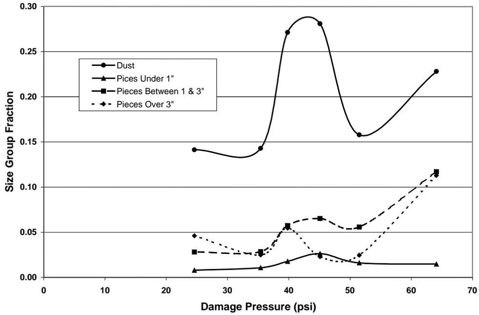
Figure II-11. Debris-Size Distributions for OPG Calcium Silicate Tests
