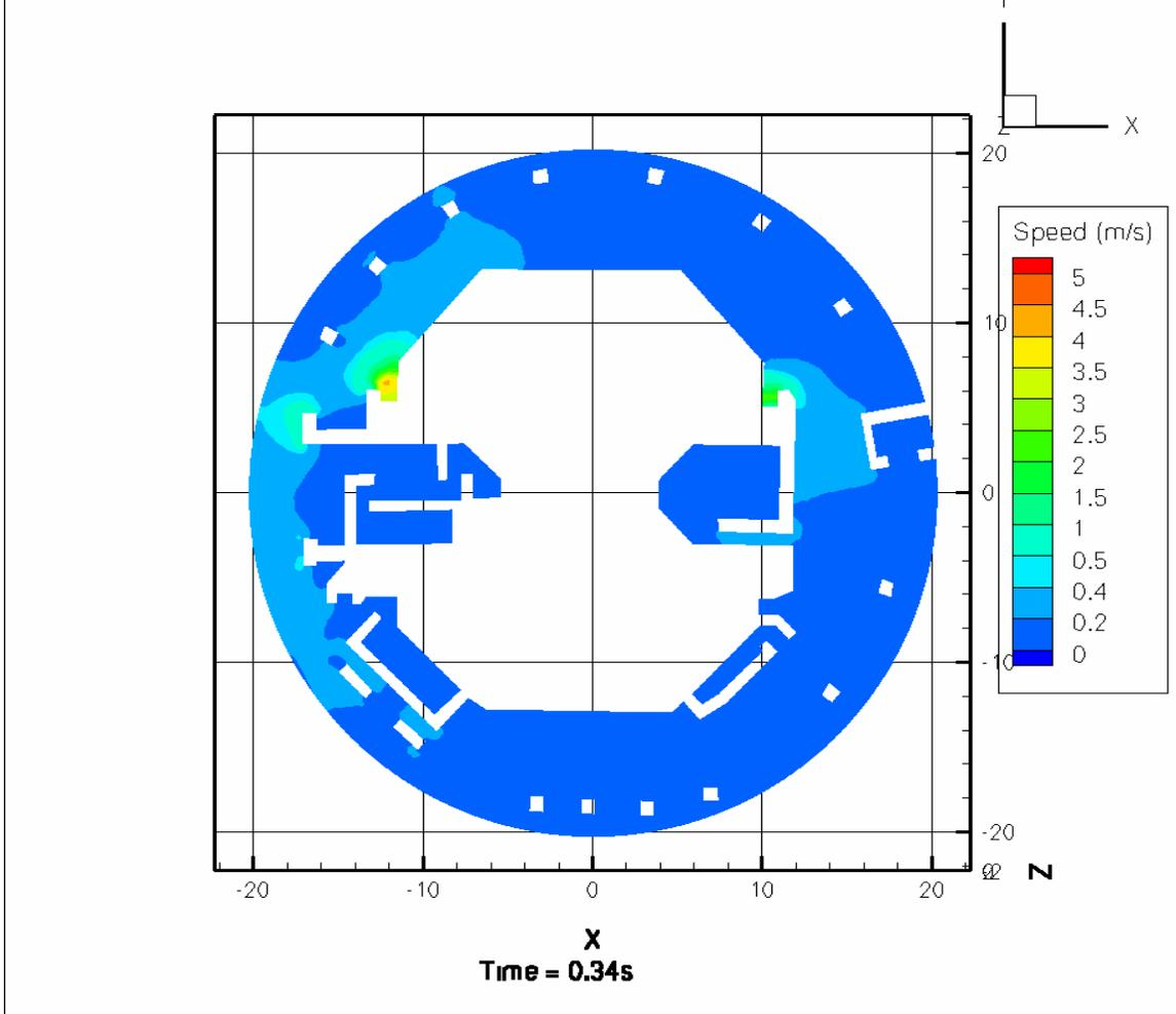
**Figure III-13. Transient VOF Simulation of Containment Pool Fillup**
