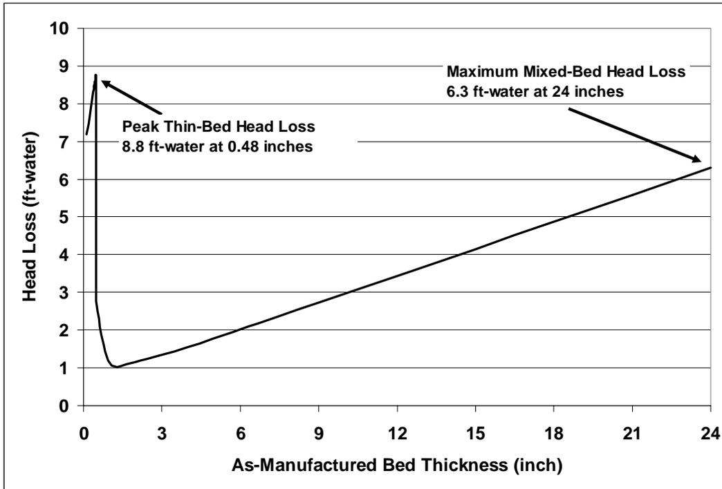
**Figure VIII-10 Specific Example of Estimating Conservative Thin-Bed Head Losses**
