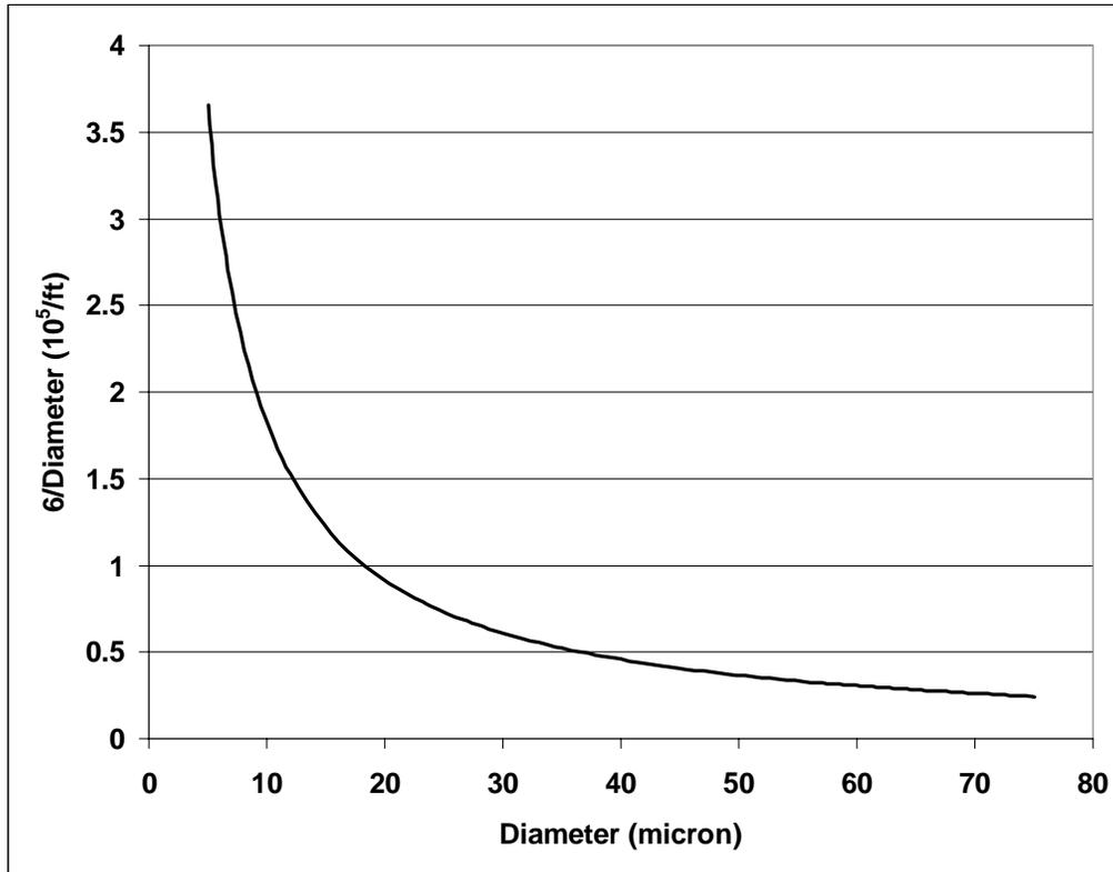
**Figure V-5. Example of Sv Variation with Particle Diameter**
