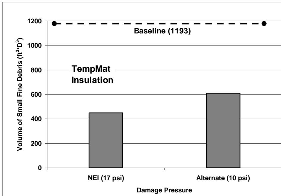
**Figure II-5. Potential Volumes of Small Fine Temp-Mat Debris**
