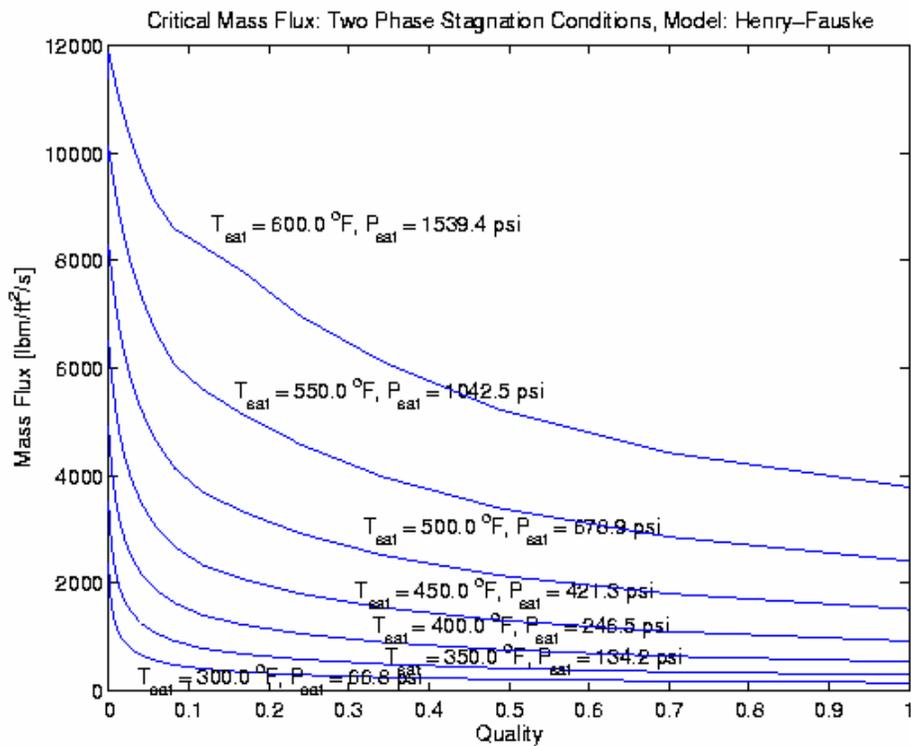
Figure I-8. Henry-Fauske Critical Mass Flux, Saturated Stagnation
