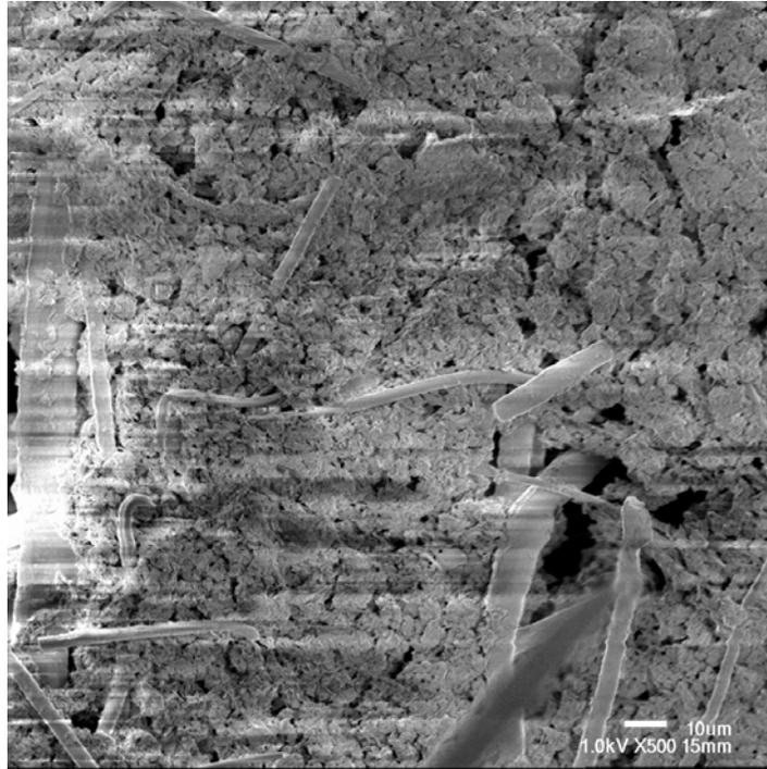
**Figure VIII-3. Posttest SEM Photo of Calcium Silicate Debris from a Thin-Bed Test**
