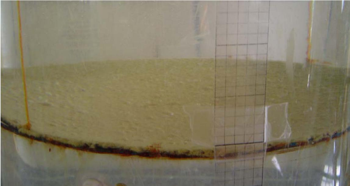
**Figure VIII-5. Debris Bed for the Calcium Silicate Head-Loss Test 6H**
