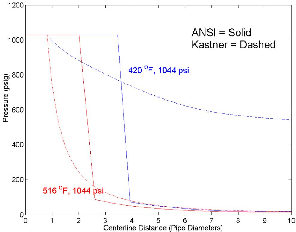
**Figure I-23. Comparison of Jet Centerline Pressure Predictions**
