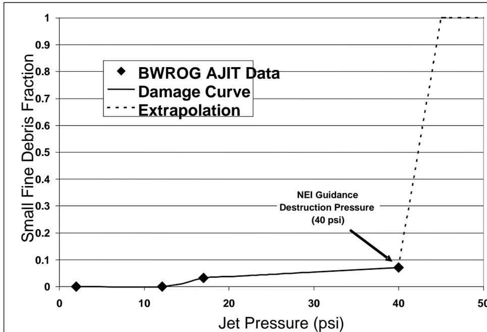
**Figure II-6. K-Wool Damage Curve for Small Fine Debris**
