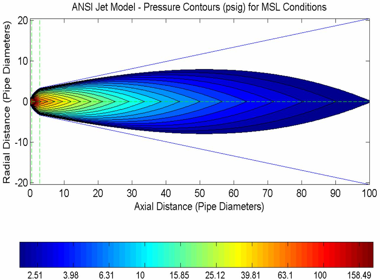
**Figure I-20. ANSI Jet-Model Stagnation Pressures for MSL Break Conditions
