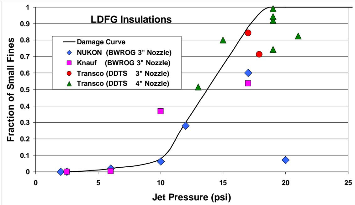
Figure II-2. LDFG Damage Curve for Small Fine Debris
