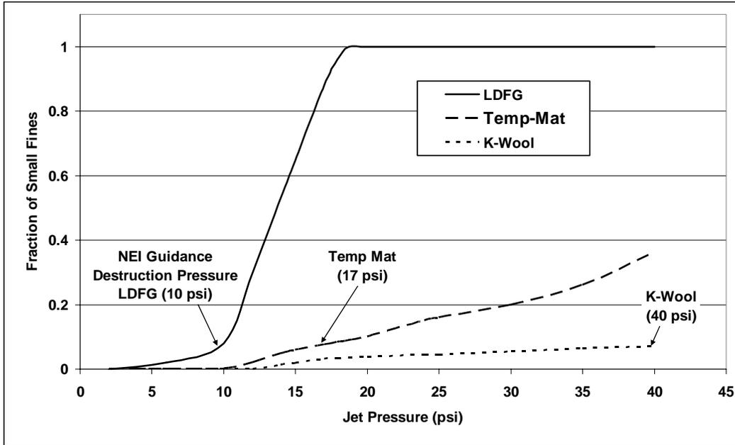
**Figure II-8. Comparison of Fibrous Insulation Damage Curves**
