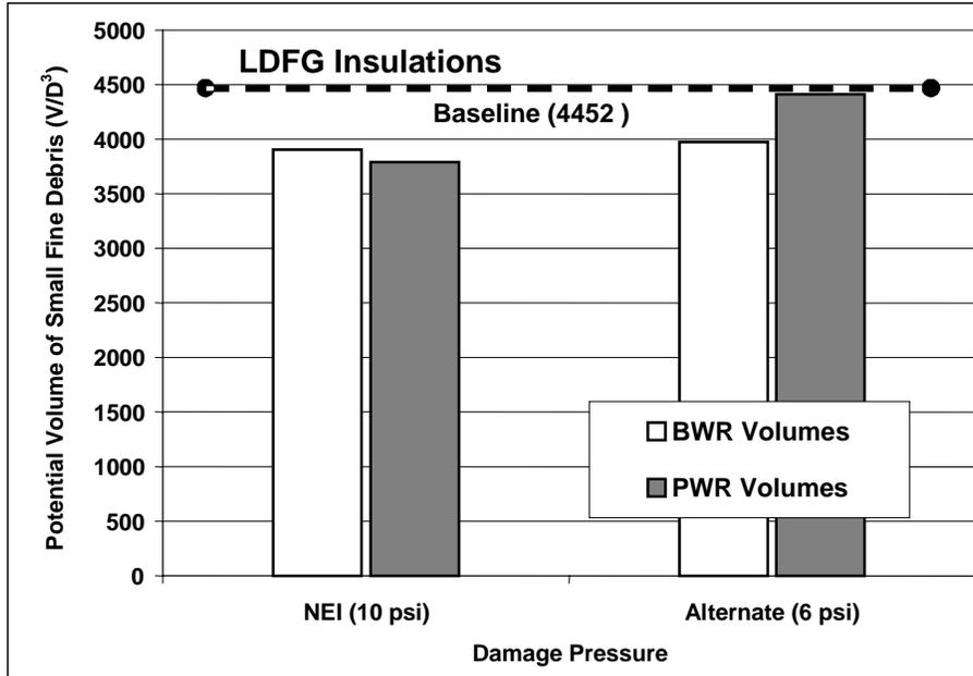
**Figure II-3. Potential Volumes of Small Fine LDFG Debris**
