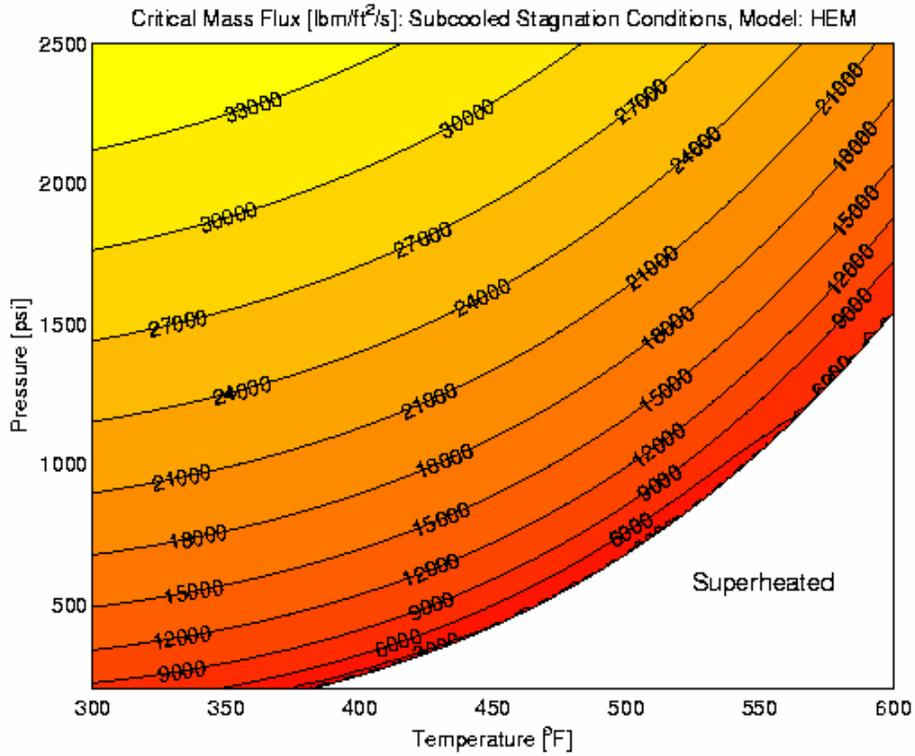
Figure I-5. HEM Critical Mass Flux, Subcooled Stagnation
