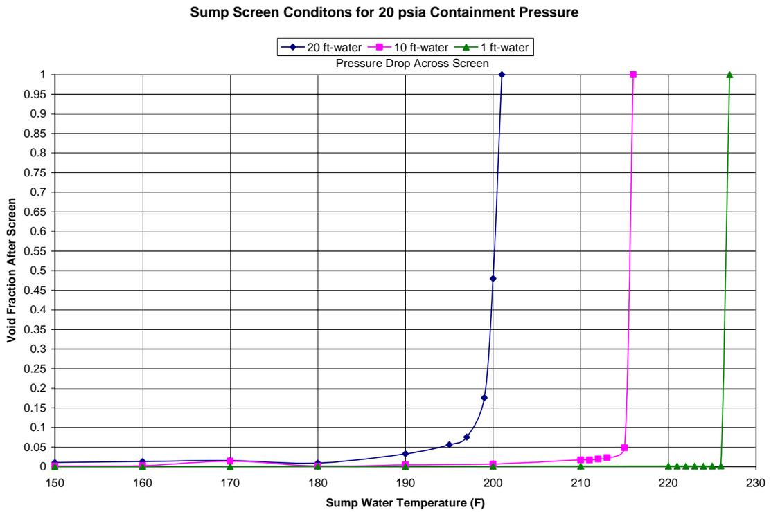
Figure 2: Downstream Void Fraction Versus Water Temperature at 20 psia
