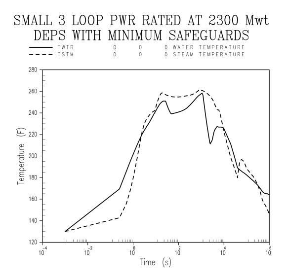
Figure 5: Three Loop Post-LOCA Temperature Profile (Logarithmic Time Scale).
