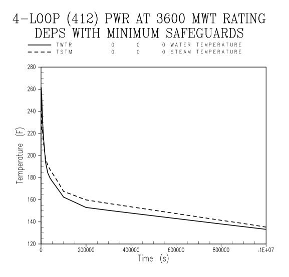
Figure 2: Four Loop Post-LOCA Temperature Profile (Linear Time Scale).
