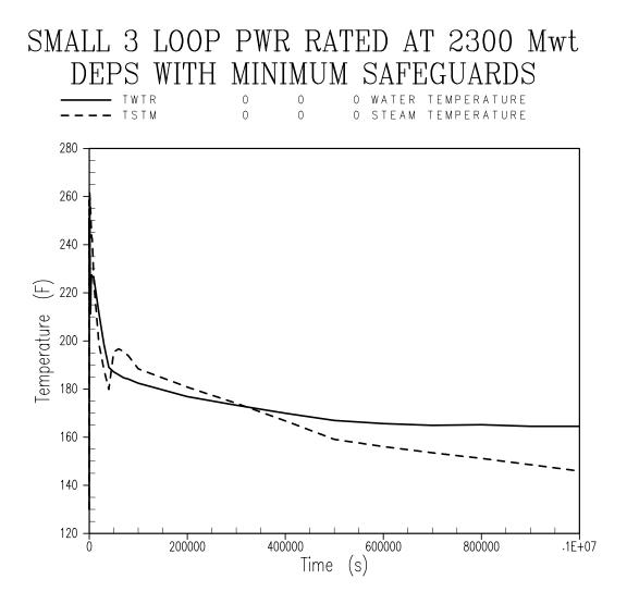
Figure 4: Three Loop Post-LOCA Temperature Profile (Linear Time Scale).
