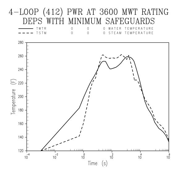
Figure 3: Four Loop Post-LOCA Temperature Profile (Logarithmic Time Scale).
