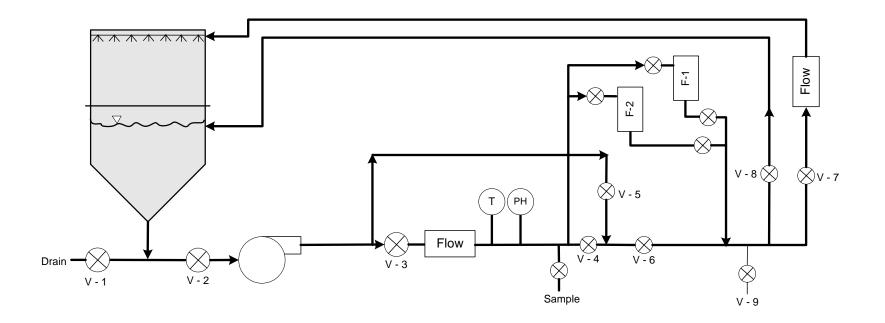
Figure 1 – Test Loop Process Flow Diagram
