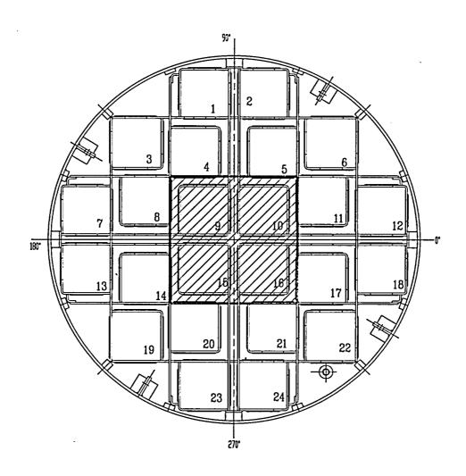
FIGURE 2.1-2 FUEL LOADING REGIONS - MPC-24E/24EF
