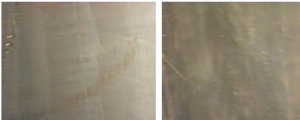
Figure 4.4 Reduction of Visual Acuity During Scanning. Left: a screen capture from when the camera is not moving. The vertical lines are sharp and the picture is relatively clear. Right: a screen capture of different area when the camera is moving. The vertical lines are blurred, as is the rest of the picture.
