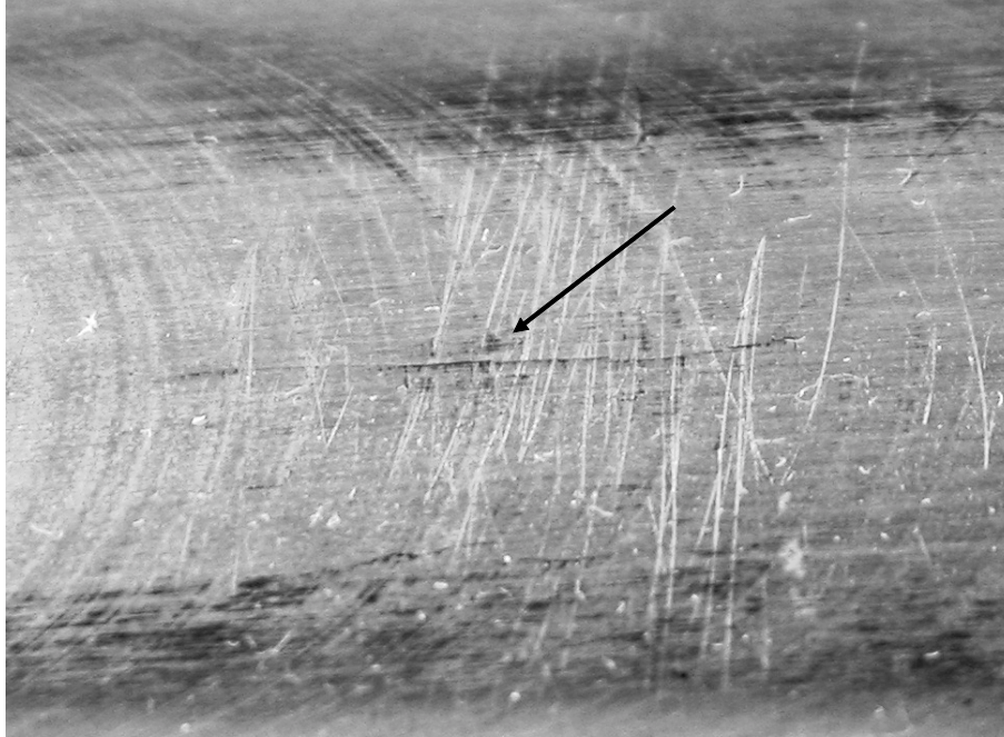
Figure 4.7 12- \mu\text{m} (0.0005-in) COD Thermal Fatigue Crack on Machined Surface. The crack is clearly visible despite its small COD, as there is discoloration around the crack opening
