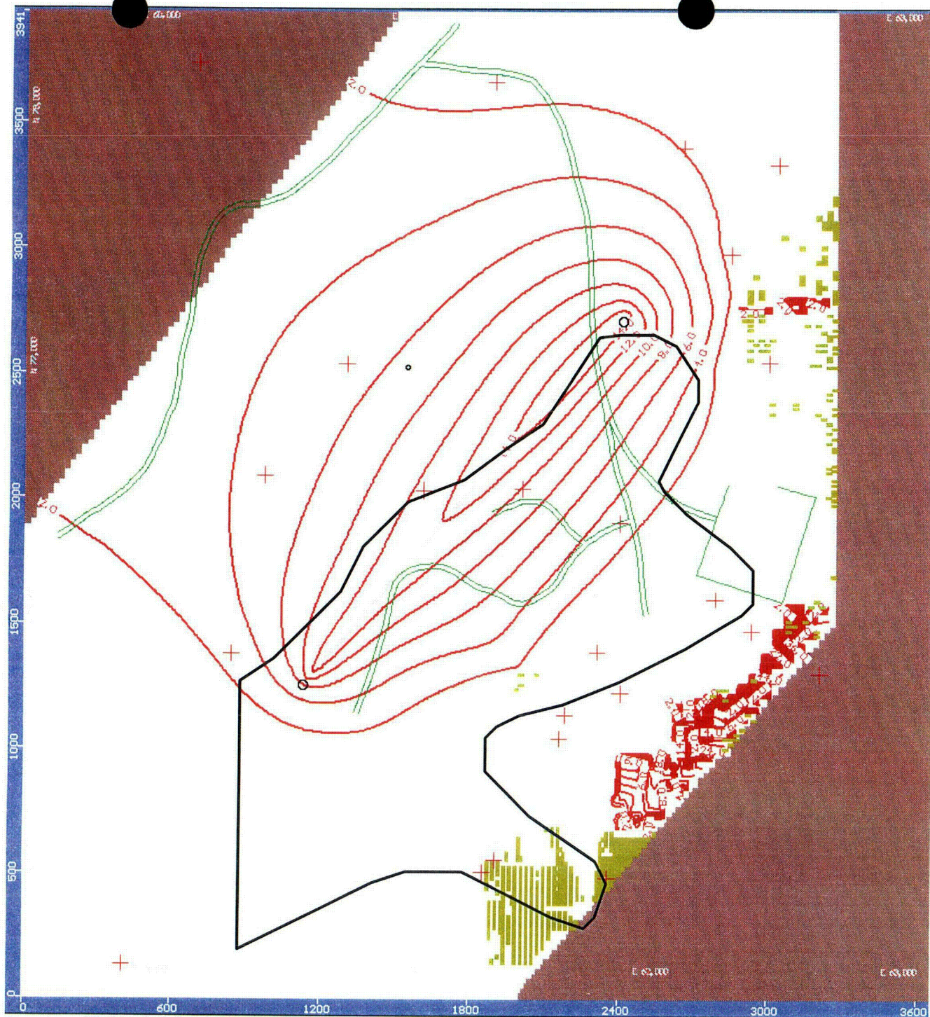
Figure 63 8. Horizontal Well Drawdown 3 Years
