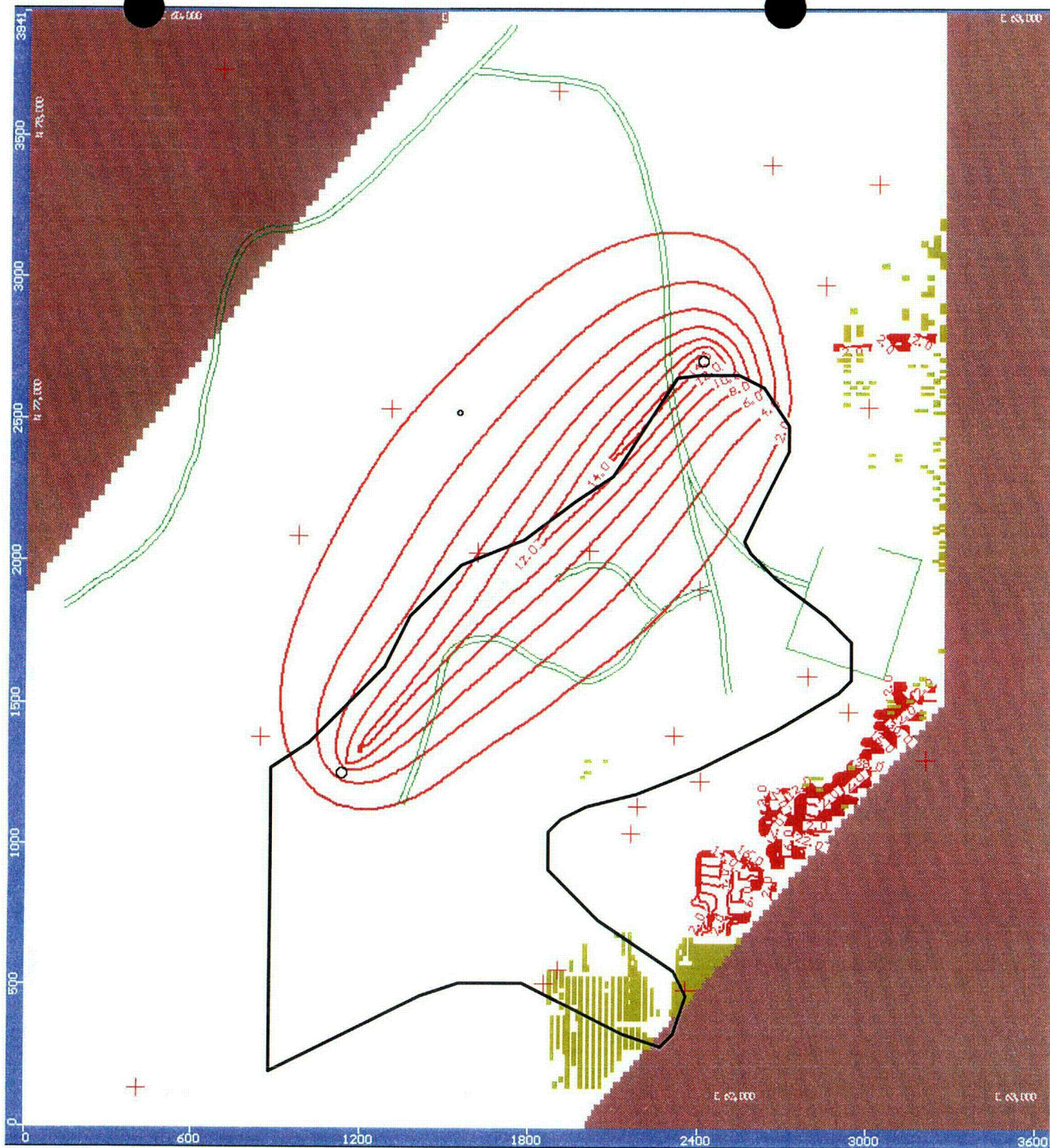
Figure 62 8. Horizontal Well Drawdown 1 Year
