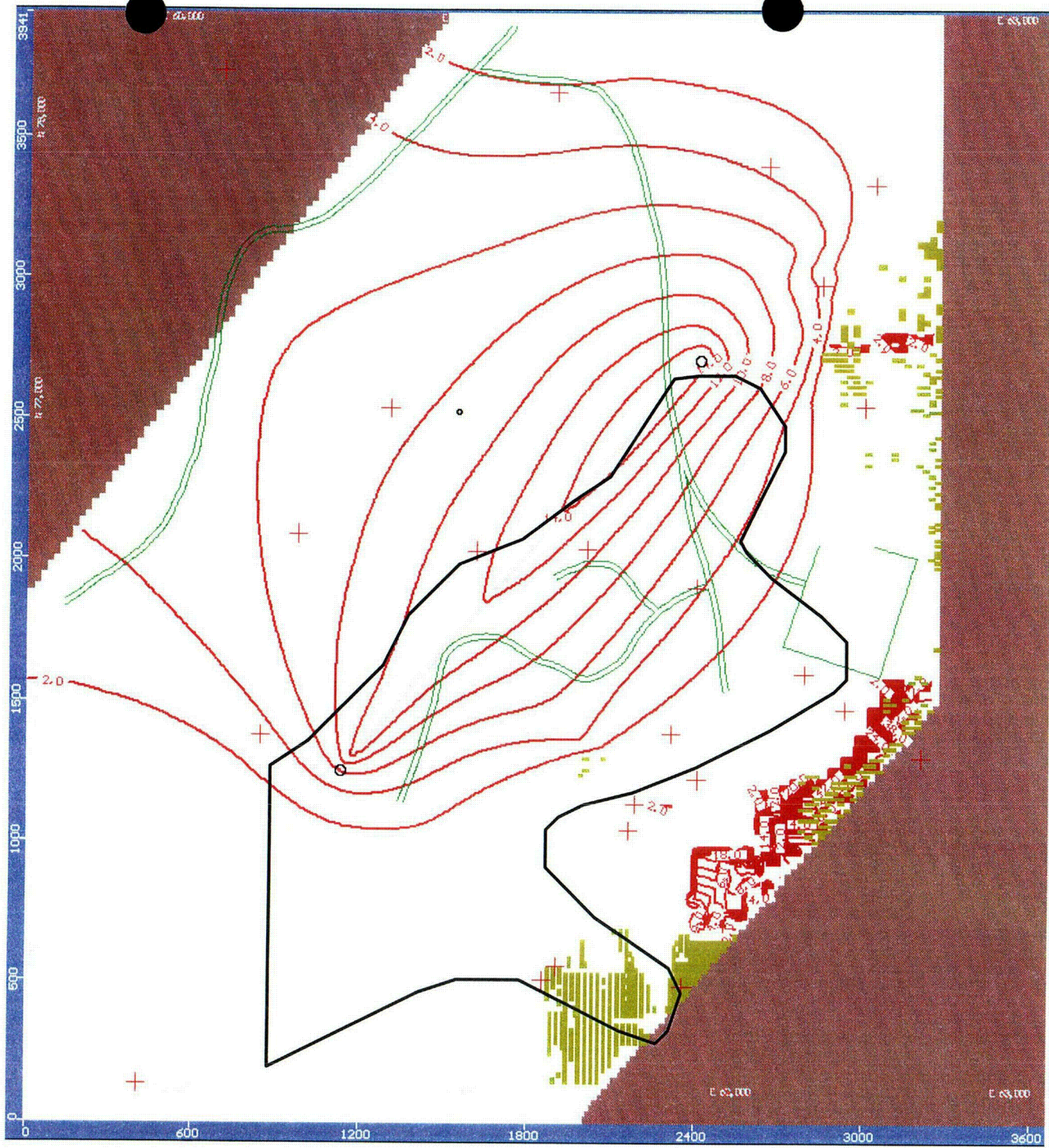
Figure 64 8. Horizontal Well Drawdown 5 Years
