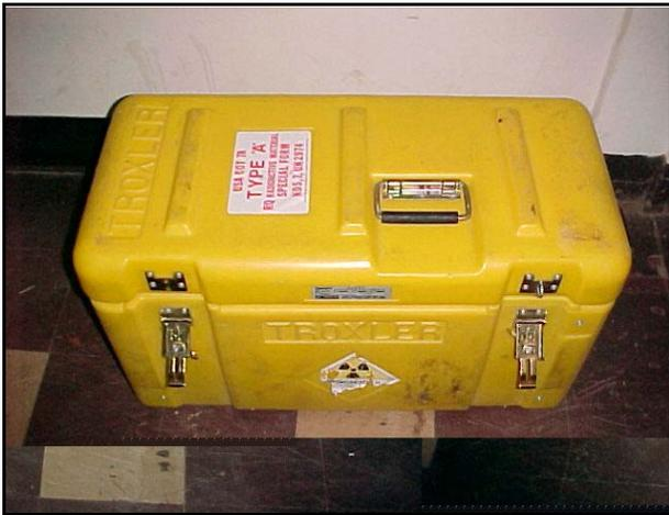
A typical carrying case for a moisture-density gauge.
