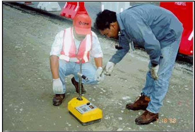
A typical moisture-density gauge in use.
