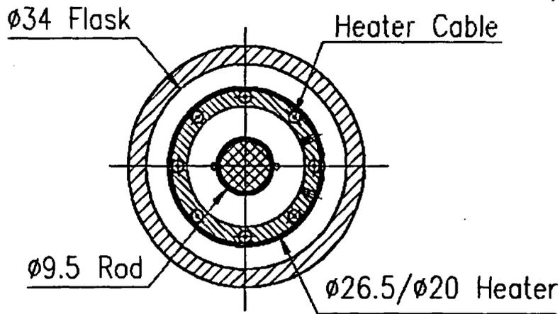
Fig. 1. The geometry of the test section
