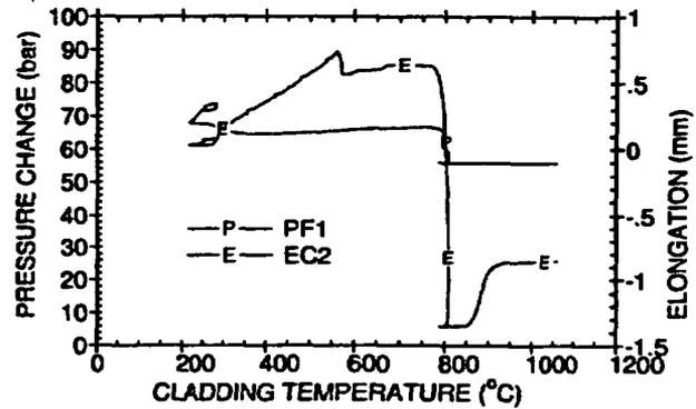
Fig. 3. Measurements of rod pressure and cladding elongation as function cladding temperature during the LOCA test (Rod rupture at 800°C)
