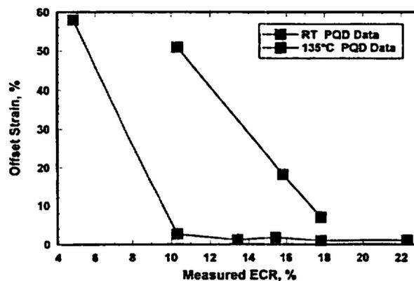
Fig. 1. Post-quench ductility of ZIRLO oxidized at 1200°C and ring-compressed at RT and 135°C.
