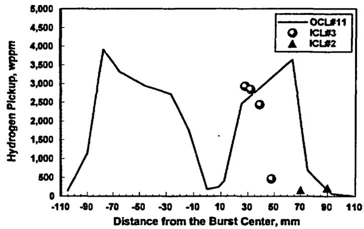
Fig 2. Axial profile of hydrogen pickup in high-burnup BWR cladding used in LOCA integral tests ICL#2 and ICL#3 (5 minutes at 1204°C); OCL#11 results are for nonirradiated Zry-2 cladding.
