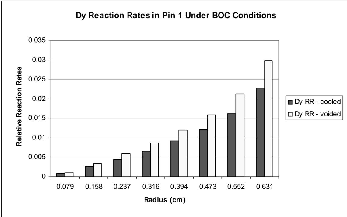
**Figure 7 Dysprosium Reaction Rates at Zero Burnup**
