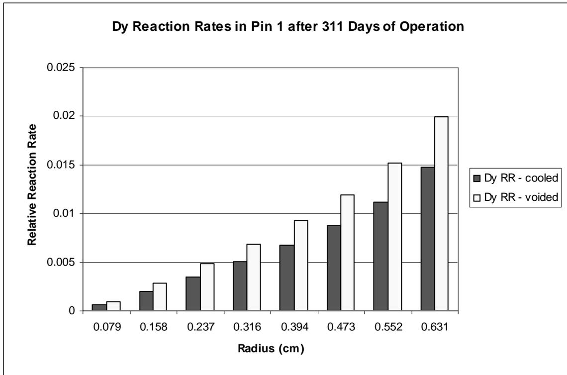
**Figure 8 Dysprosium Reaction Rates at 311 Days**
