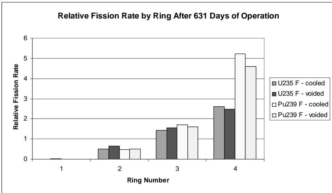
**Figure 6a Relative Reaction Rates at 631 Days - Fission**
