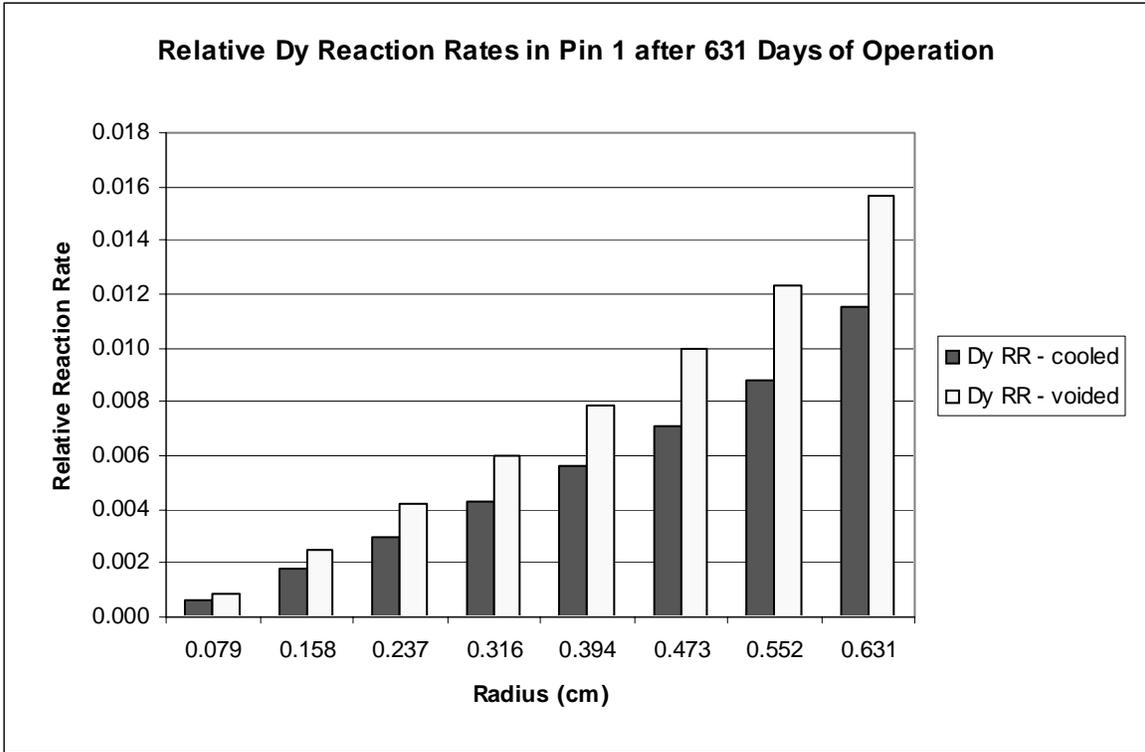
**Figure 9 Dysprosium Reaction Rates at 631 Days**
