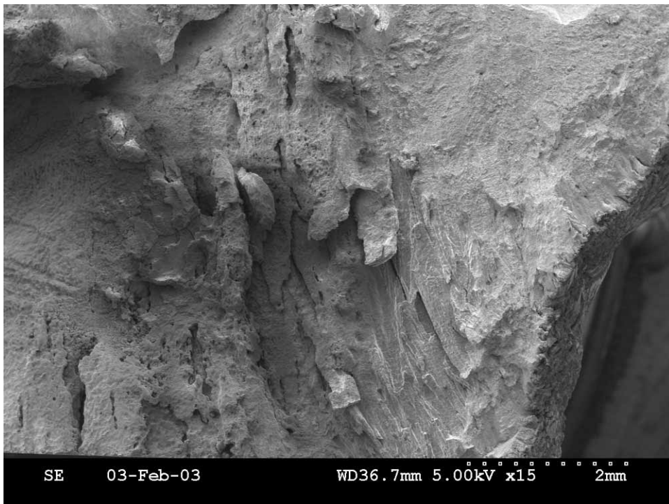
Figure 7.2.4.5: Higher magnification of the right section in Figure 7.2.4.2. Cracking to the left side of ductile tearing (lab fracture) is interdendritic.
