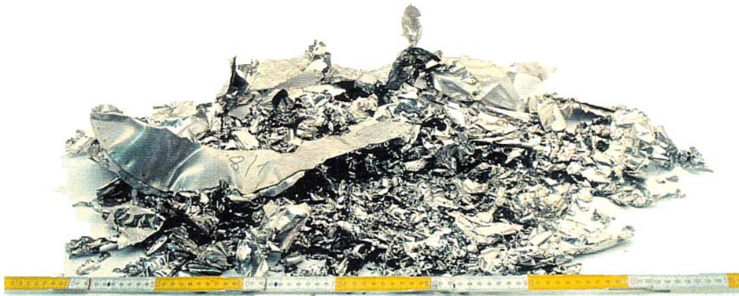
Figure IX-3. RMI Debris Observed in Siemens Steam-Jet Impact Tests.
