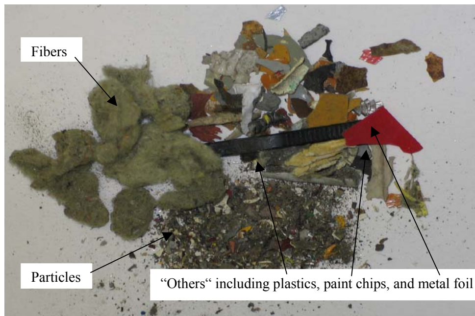
Figure VII-1. Representative Latent-Debris Components from a Single Volunteer Plant.
