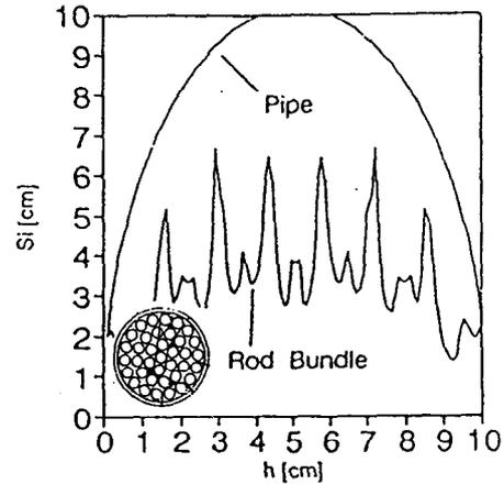
Figure 4: Interfacial Length for 37-Rod Bundle.
