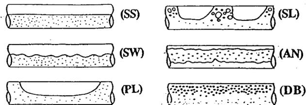
Figure 1 : Flow Regimes in a Horizontal Pipe
