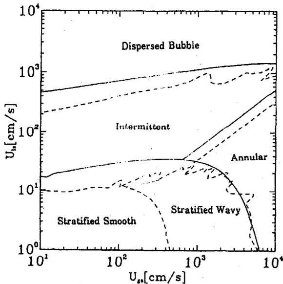
Figure 3 Predicted Flow Regime Map for 37-Rod Bundle Geometry ( $D = 10.16$  cm I.D., Pin Diameter,  $d = 1.27$  cm) and a 10.16 cm I.D. Pipe at Room Temperature,  $T = 25^\circ\text{C}$  and Pressure,  $P = 1.01$  bar.
