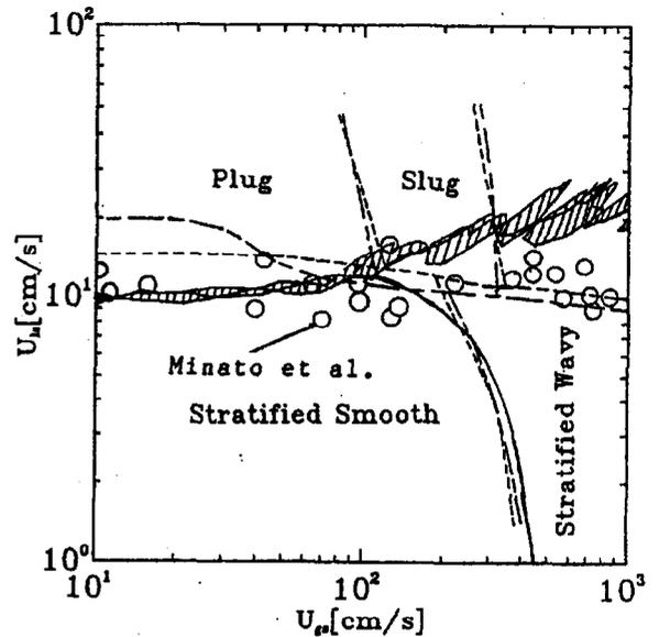
Figure 6 Comparison of Present Results with the Data of Minato et al.<sup>7</sup> for a 37-Rod Bundle Geometry at Room Temperature and Pressure,  $P = 1.01$  bar.
