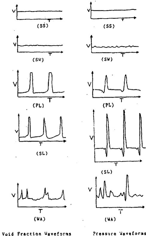
Figure 1b Pressure Drop and Void Fraction Signal Waveforms for 37-Rod Bundle Flow Geometry
