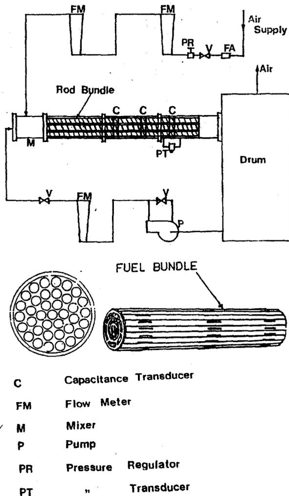
Figure 2 Schematics of Experimental Loop.
