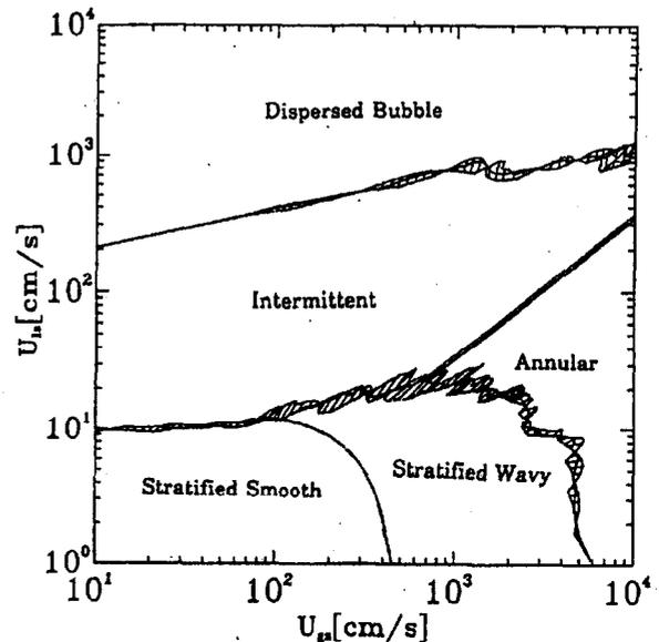
Figure 4 Calculated Flow Pattern Transitions for 37-Rod Bundle Geometry at Different Angles of Orientation.
