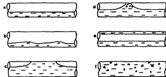
Figure 1a Flow regimes in Horizontal Two-Phase Flow
