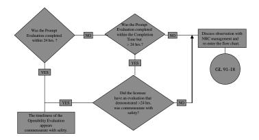
The 24 hour guidance is for SSCs in TS and is subsequent to immediately declaring a system operable/inoperable. The 24 hour guidance is not a grace period to be utilized for repair of a degraded or non-conforming condition (i.e. it is not a 24 hour extension of the Completion Time).
