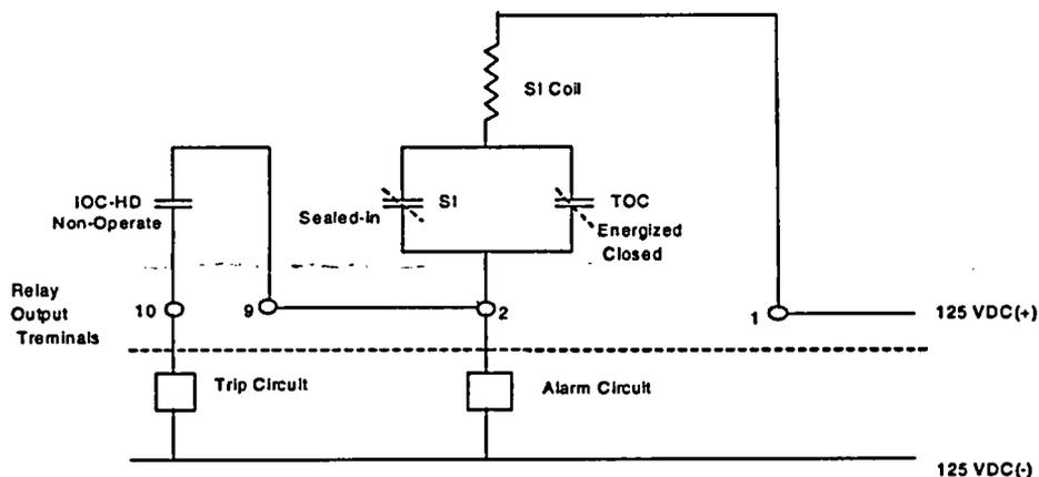
Figure 1 IAC66K Relay Internal Configuration
