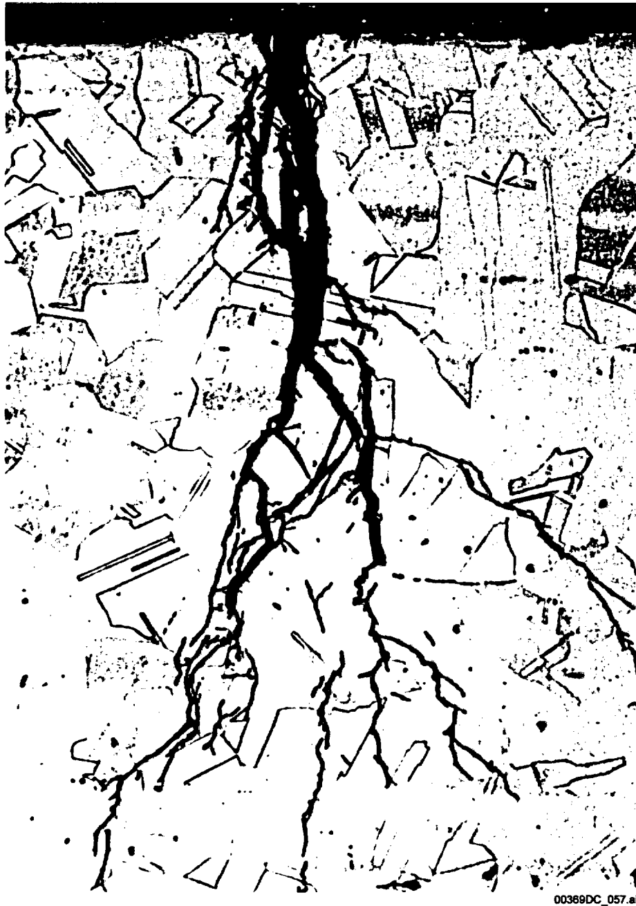
Figure 5-3. Typical Example of Transgranular Stress Corrosion Cracking in Stainless Steel
