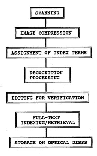
Figure 1 - Flow Diagram of Image Archive and Full-text Retrieval System
