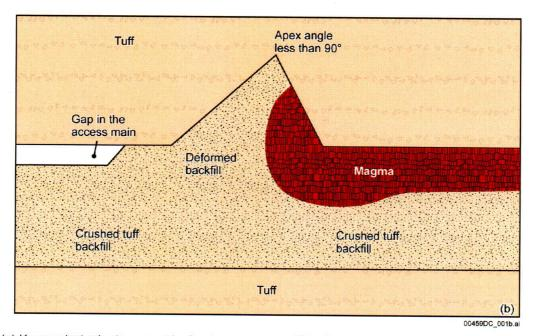
NOTE: (a) Keyway just prior to contact by flowing magma and (b) after contact with magma showing deformation of fill and closure of the open space in the keyway.
