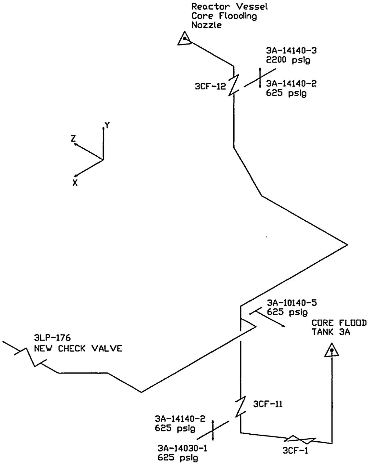
Figure 1-2 Isometric View of Oconee Unit 3 - Train B CF/LPI/DHR Piping System
