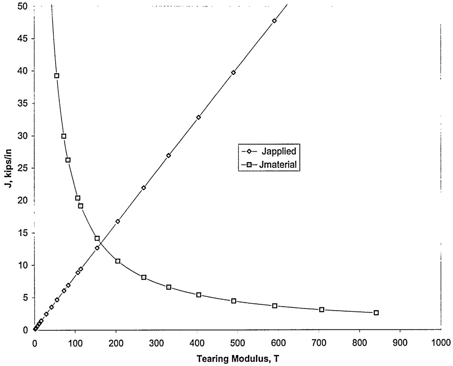
Figure 7-8 J versus T diagram for SMAW Weld Metal at LBB Location 2
