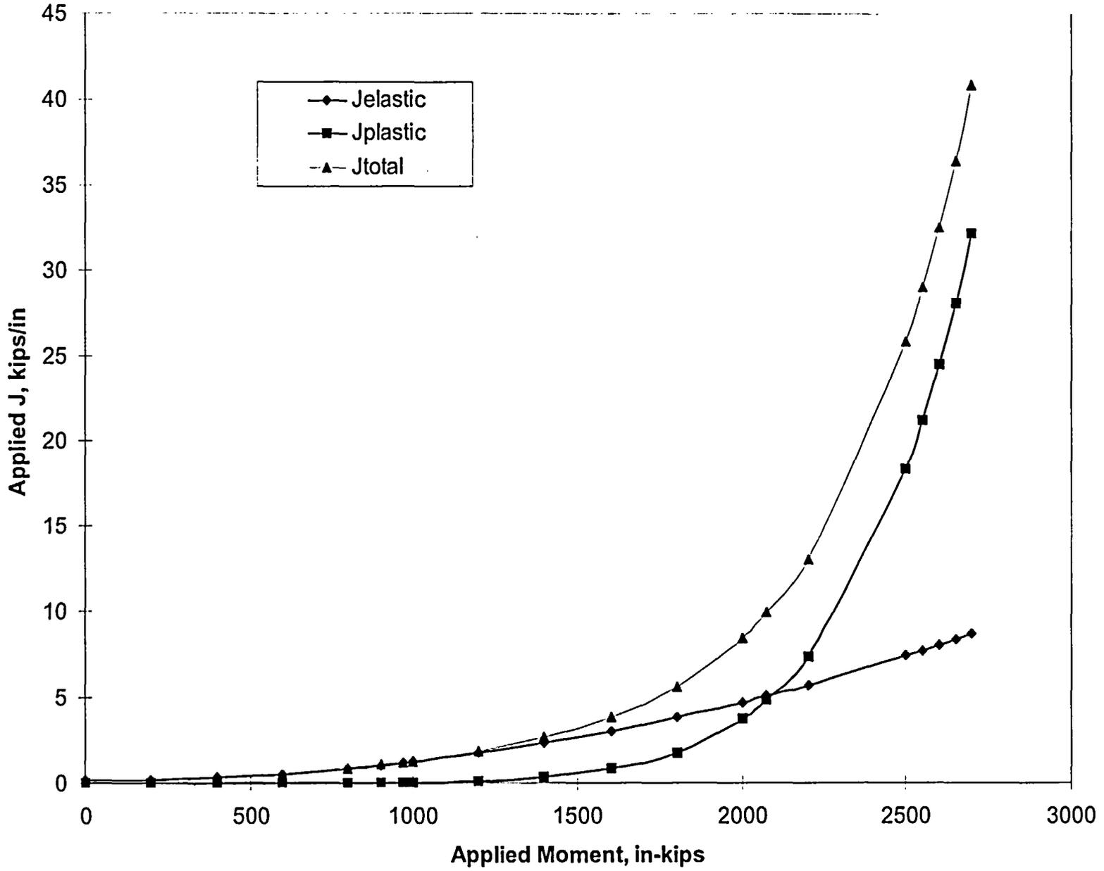
Figure 7-2 Illustration of J versus Applied Moment Loading Diagram
