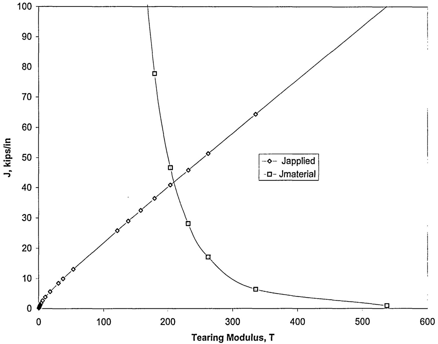
Figure 7-6 J versus T diagram for Type 316SS Base Metal at LBB Location 2
