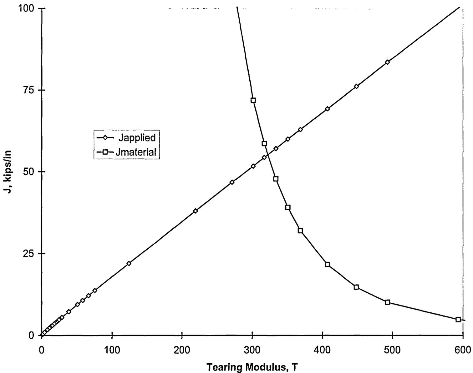
Figure 7-5 J versus T diagram for GTAW Weld Metal at LBB Location 1
