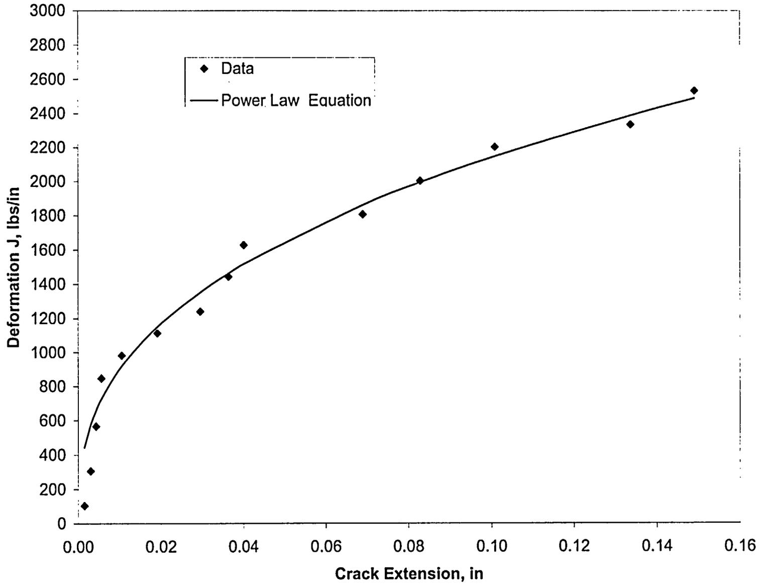
Figure 3-6 J-R Curve for SMAW Weld Metal at 550°F
