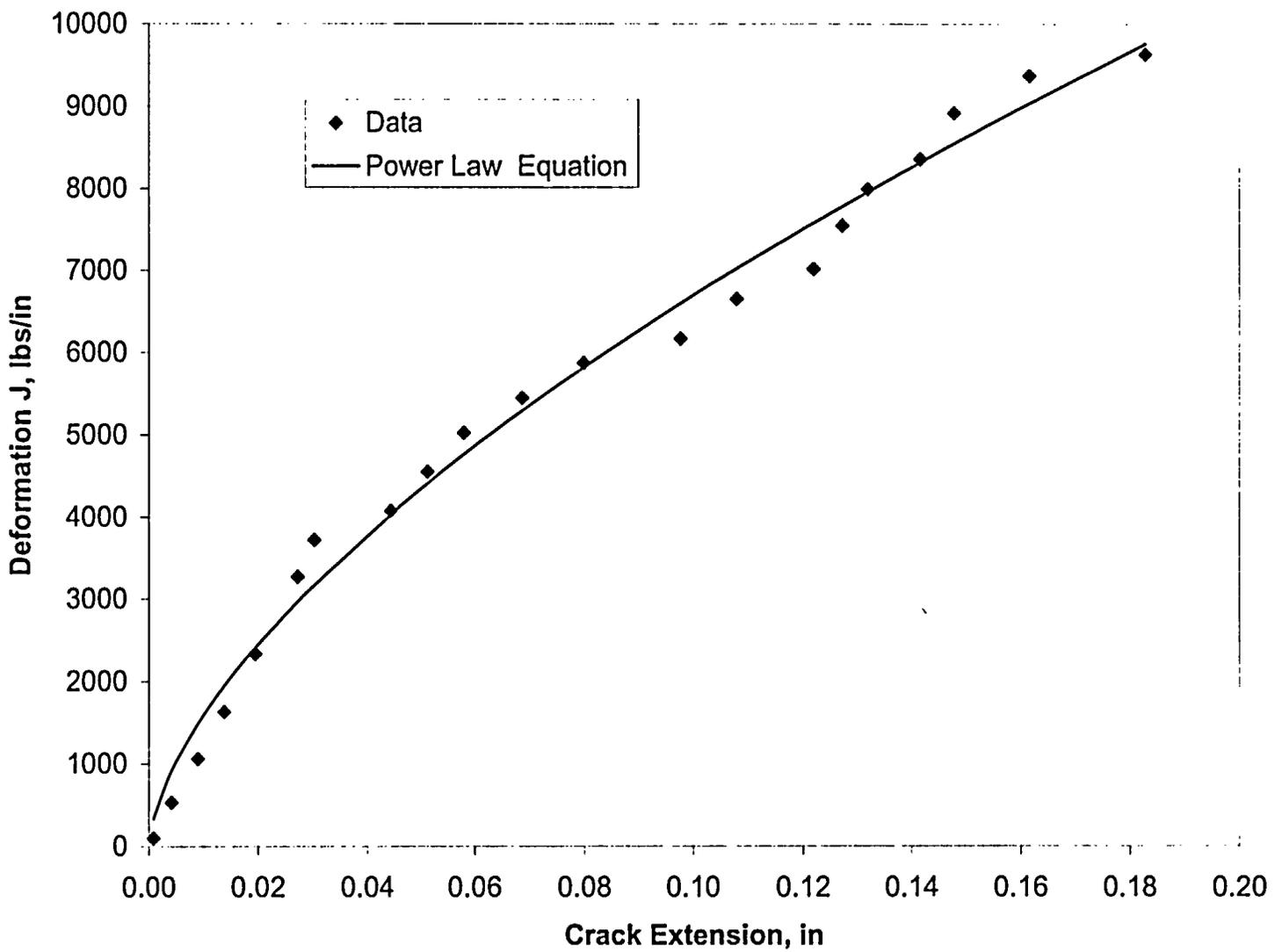
Figure 3-5 J-R Curve for Type 304SS Base Metal at 550°F
