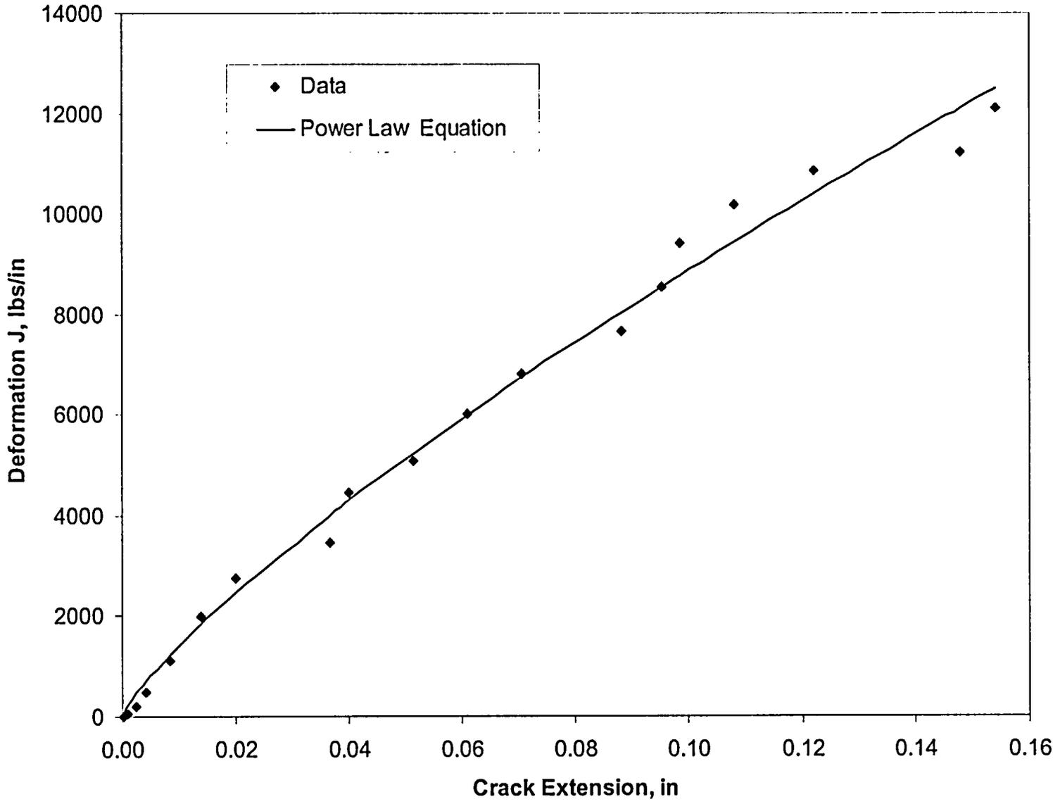
Figure 3-3 J-R Curve for GTAW Weld Metal at 75°F
