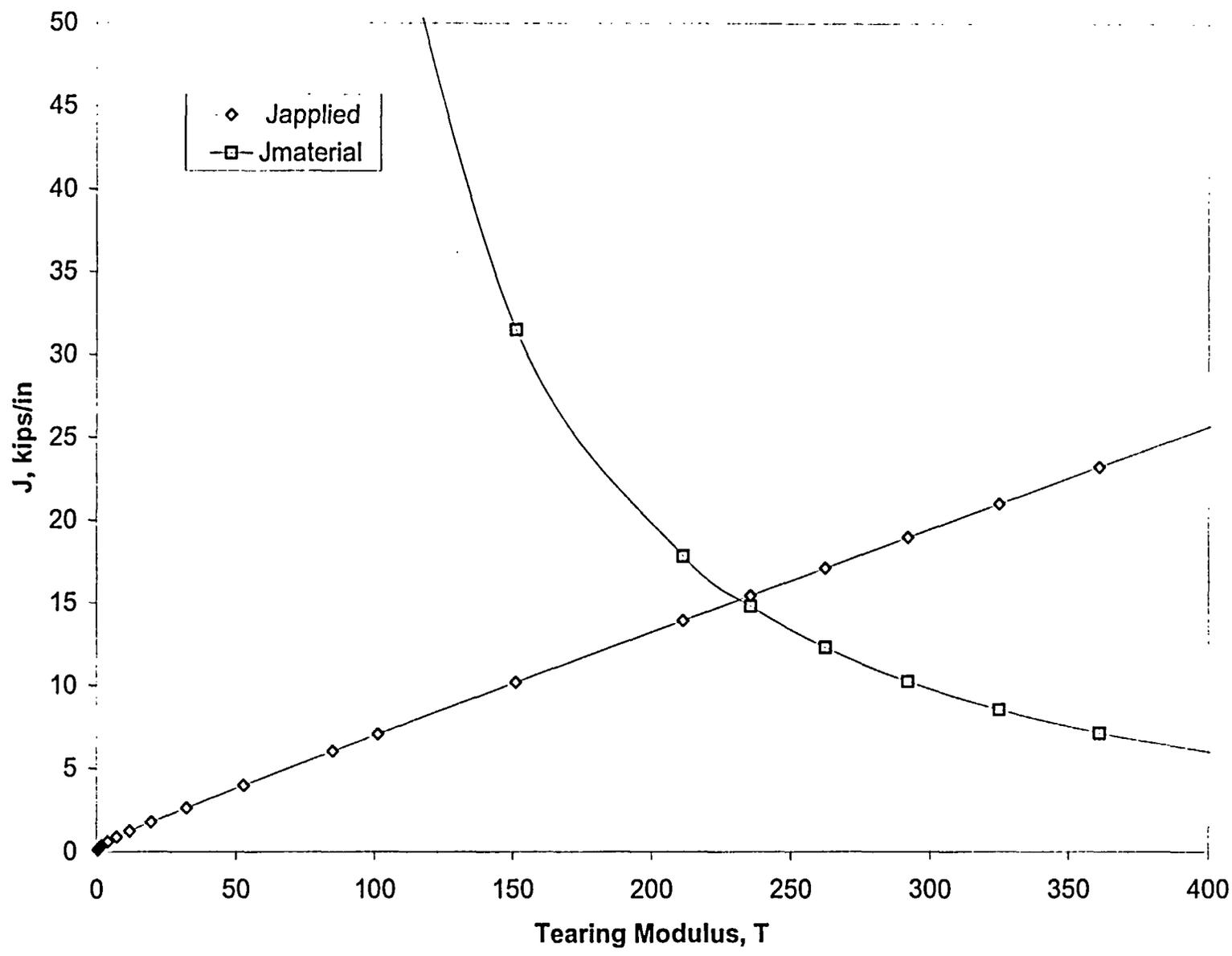
Figure 7-7 J versus T diagram for Type 304SS Base Metal at LBB Location 2
