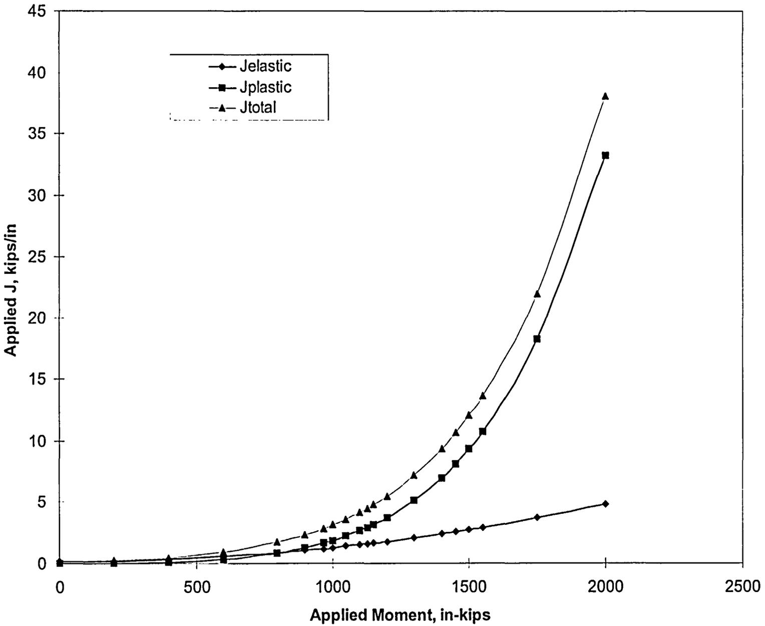
Figure 7-4 J versus T diagram for Type 304SS Base Metal at LBB Location 1
