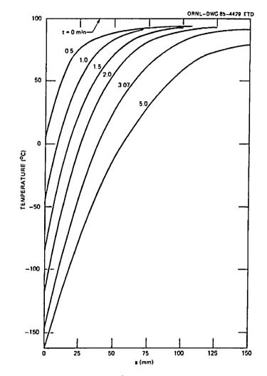
Fig. 9.6. Temperature vs a/w for several times during the TSE-5A transient.
