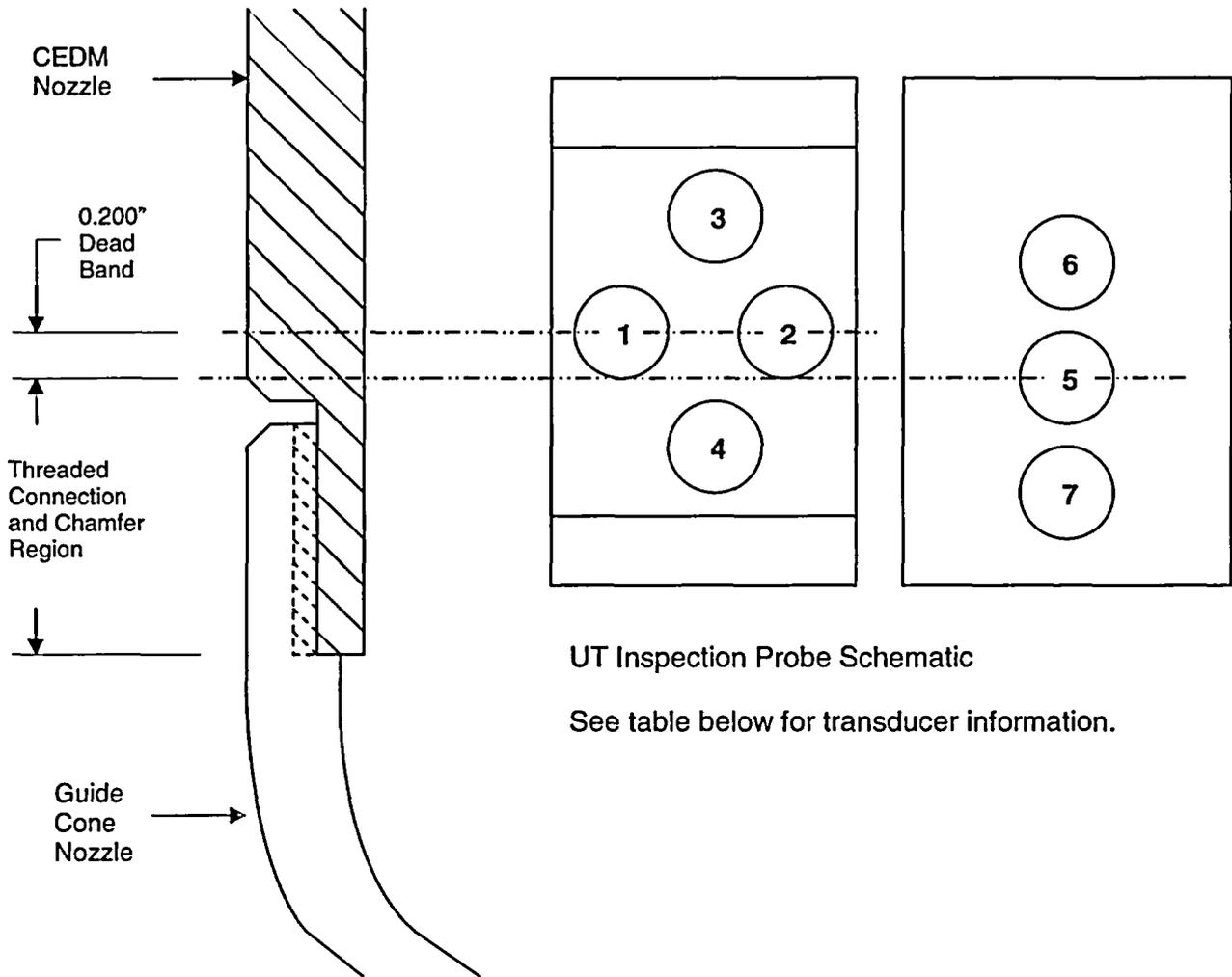
UT Inspection Probe Schematic
