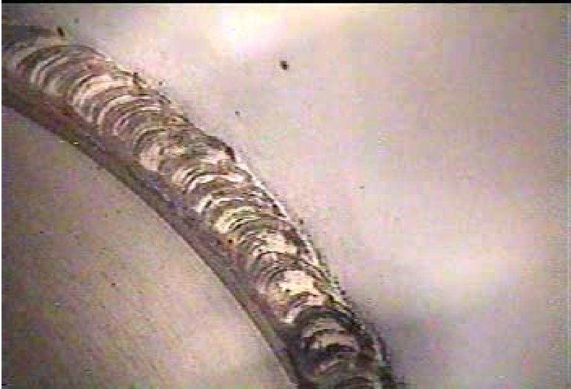
**Figure 16.2: Beam tube Number 5 (BT-5) Weld**
