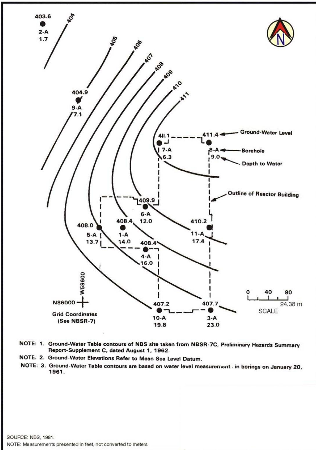
Figure 2.13: Groundwater Contour at NBSR Site
