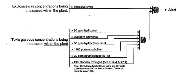
Entry of toxic or flammable gases into vital areas with plant not in Mode 5, Cold Shutdown.
