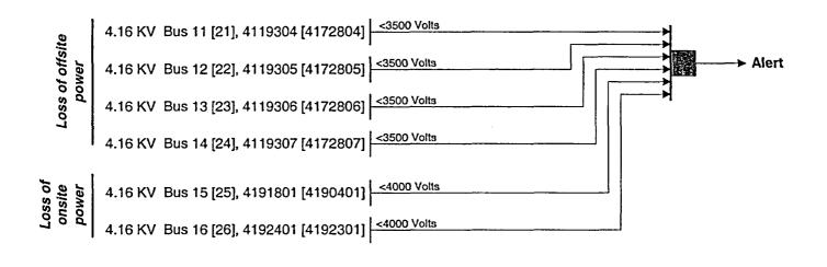
Loss of offsite power and loss of onsite. AC power for more than 15 minutes.
