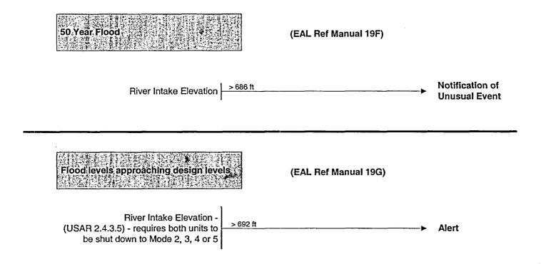
Flood levels exceeding design levels with plant not in Mode 5, Cold Shutdown
