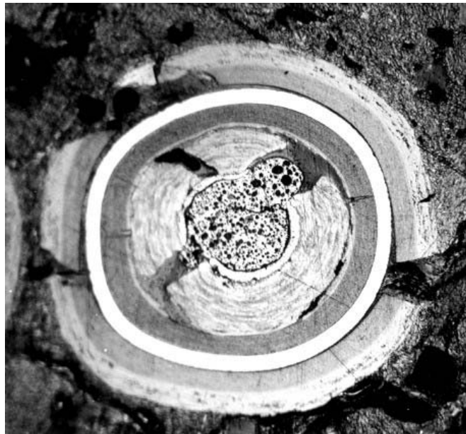
Figure 2-10 An example of a distorted buffer layer (HRB-21). (DOE-HTGR-100229)
