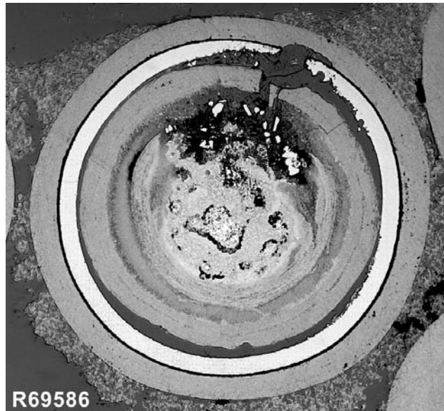
Figure 2-12 CO oxidation of SiC (WAR UO 2 kernel at ~1500°C in HRB-10)
