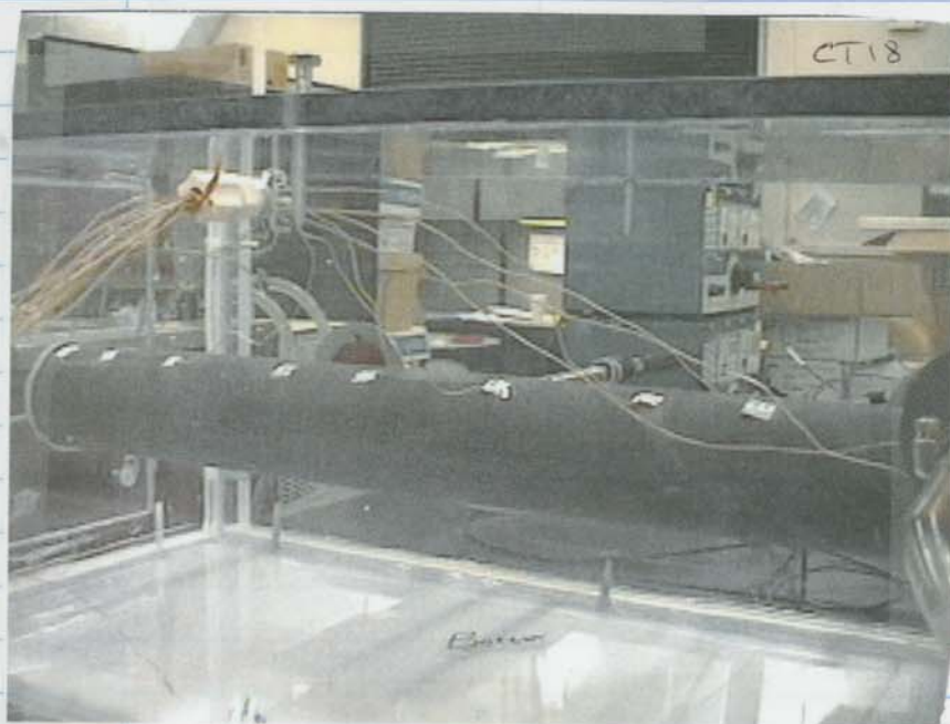
Photo showing placement & location of thin wire thermocouples along ceramic tube.
