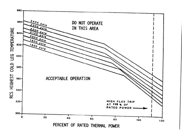
NOTE: BASED ON A MINIMUM RCS FLOW OF  $97.3 \times 10^6$  lbm/hr
