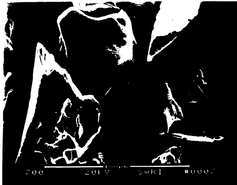
Figure 2-2. Scanning electron photomicrographs of analcime powder (230-325 mesh size): (a) before and (b) after ultrasonic cleaning
