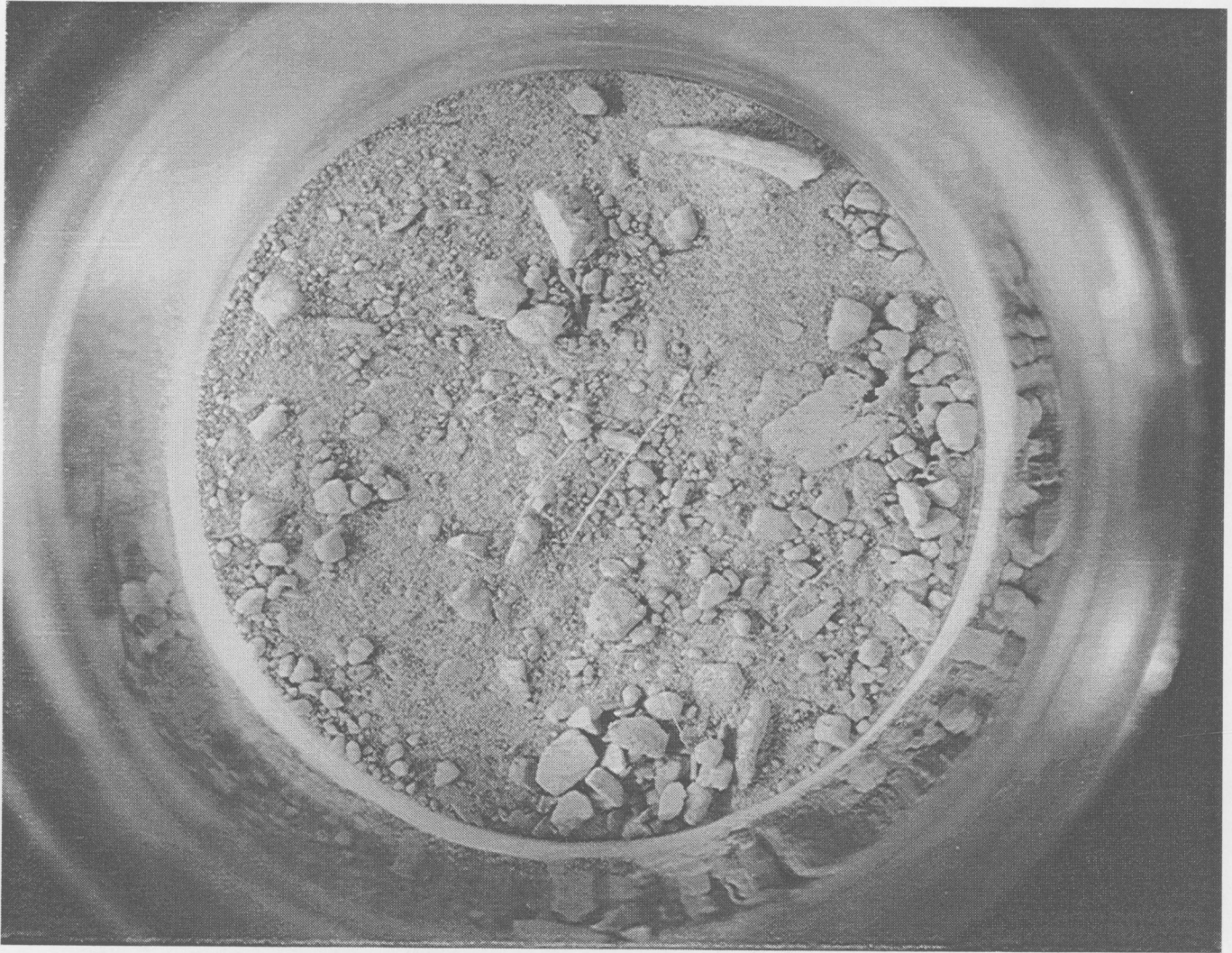
Figure 3-24. Gouge material after being dried to demonstrate texture and particle size
