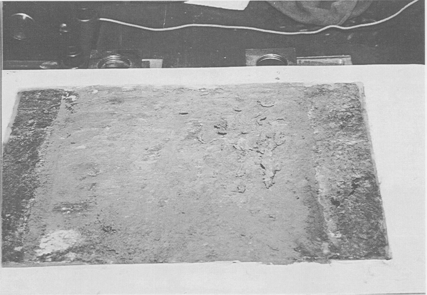
Figure 3-22. The paste-like gouge material formed during shear displacement
