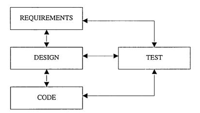
Traceability analysis ensures completeness, that all lower level requirements and design features are derived from higher level requirements, and that all higher level requirements are allocated to lower level requirements, design features, and tests. Traceability analysis is also used in managing change and provides the basis for test planning.
