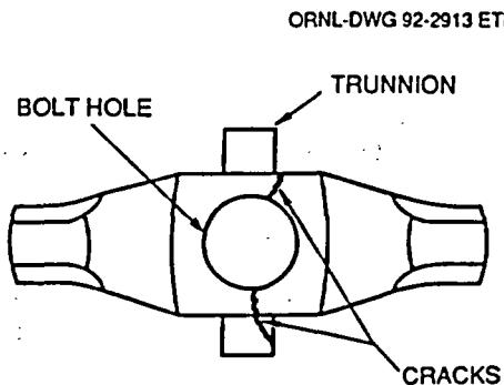
Figure 5.1 Crack locations of JET pump holddown beams
