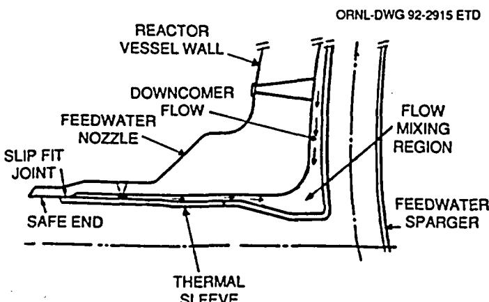
Figure 5.3 Feedwater sparger and feedwater nozzle connection
