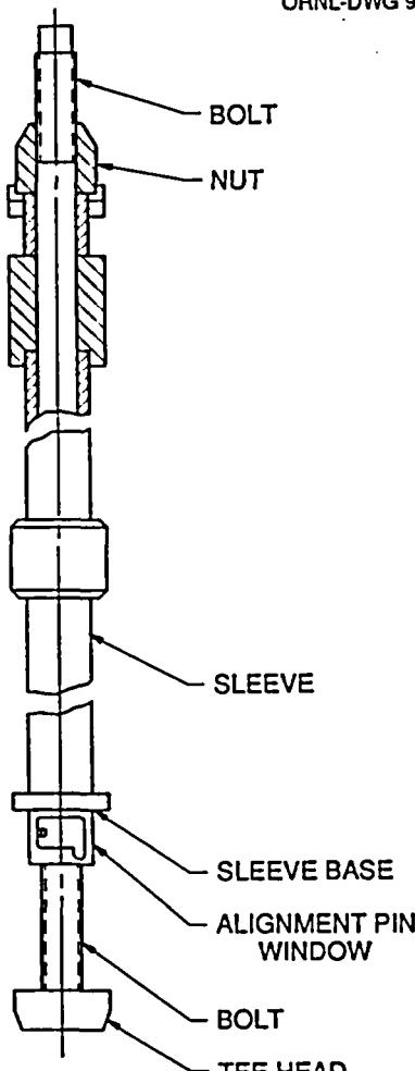
Figure 2.5 Shroud head bolt
