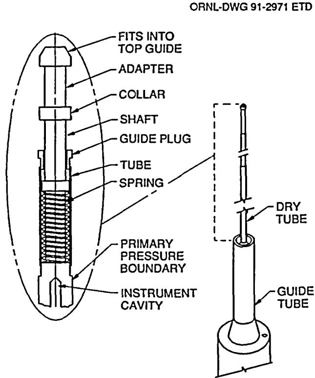
**Figure 2.15** In-core neutron flux monitor dry tube
