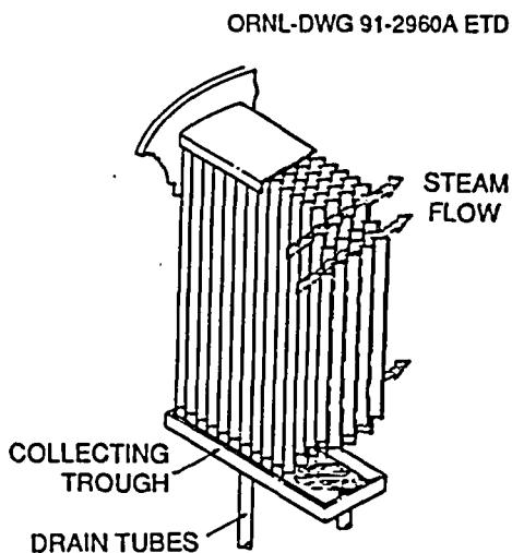
Figure 2.2 Steam dryer assembly
