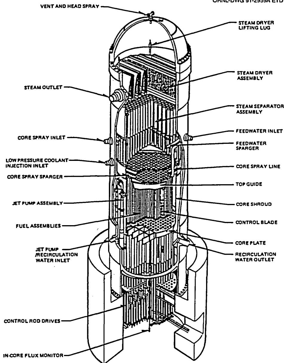
Figure 2.1(a) BWR internals with jet pumps
