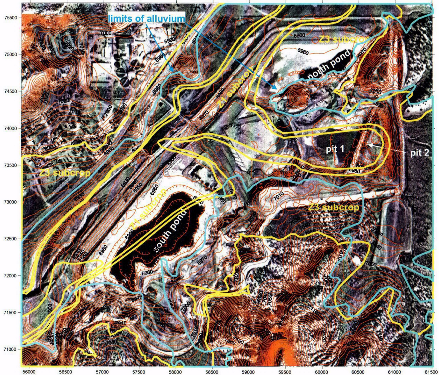
FIGURE 3 Topography and geology (after Canonie, May 1987) on circa 1983 aerial photograph of tailings ponds (5-foot contour interval)
