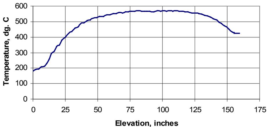
Figure 2 Axial Temperature Profile Used to Calculate Fuel Rod Pressures and Stresses
