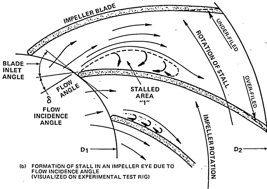
(b) FORMATION OF STALL IN AN IMPELLER EYE DUE TO FLOW INCIDENCE ANGLE (VISUALIZED ON EXPERIMENTAL TEST RIG)
