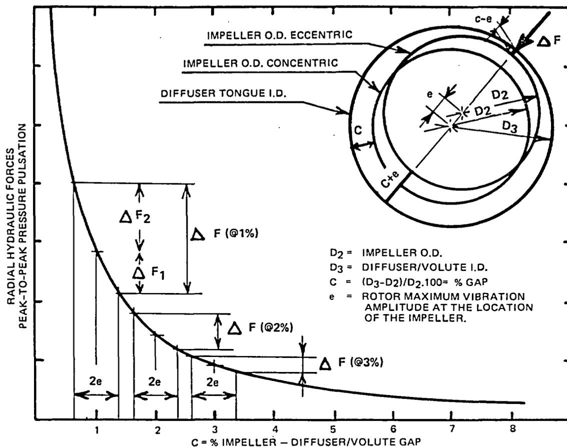
Fig. D.5. Influence of pump impeller to diffuser/volute radial gap on pressure pulsation at blade-passing frequency and rotor deflection caused radial forces. Source: R. Makay and O. Szamody, *Survey of Feed Pump Outages*, EPRI FP-754, Electric Power Research Institute, April 1978.
