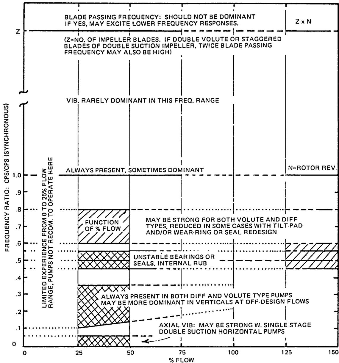
Fig. D.6. Frequencies of hydraulically induced dynamic forces acting on the rotor of a centrifugal pump. Source: E. Makay and O. Szamody, *Survey of Feed Pump Outages*, EPRI FP-754, Electric Power Research Institute, April 1978.
