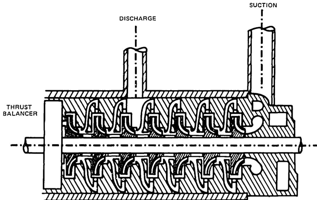
Fig. 3. Single-suction, in-line-impellers AUXFP.
