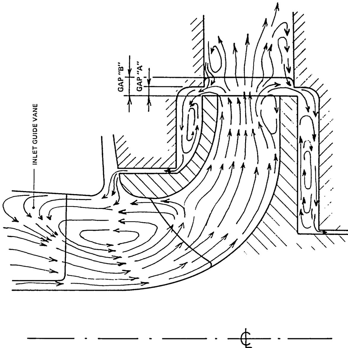
Fig. D.3. Secondary flow pattern in and around pump impeller stage at off-design flow operation. Source: E. Makay and O. Szamody, *Survey of Feed Pump Outages*, EPRI FP-754, Electric Power Research Institute, April 1978.
