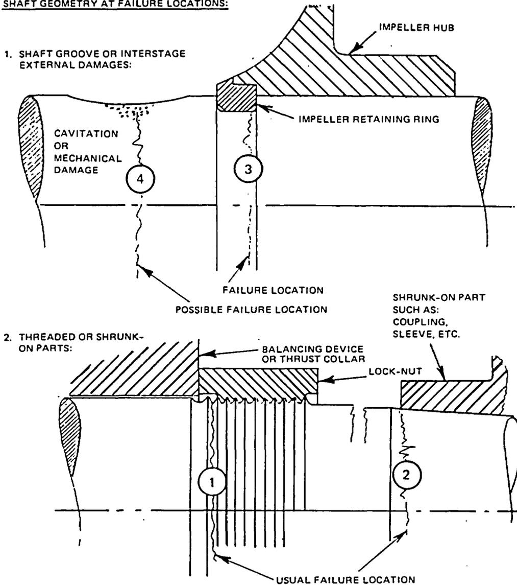
Fig. D.13. Typical multistage centrifugal pump shaft failure locations. The four most frequent locations are shown in order of failure frequency. Source: E. Makay and O. Szamody, *Recommended Design Guidelines for Feedwater Pumps in Large Power Generating Units*, EPRI CS-1512, Electric Power Research Institute, September 1980.
