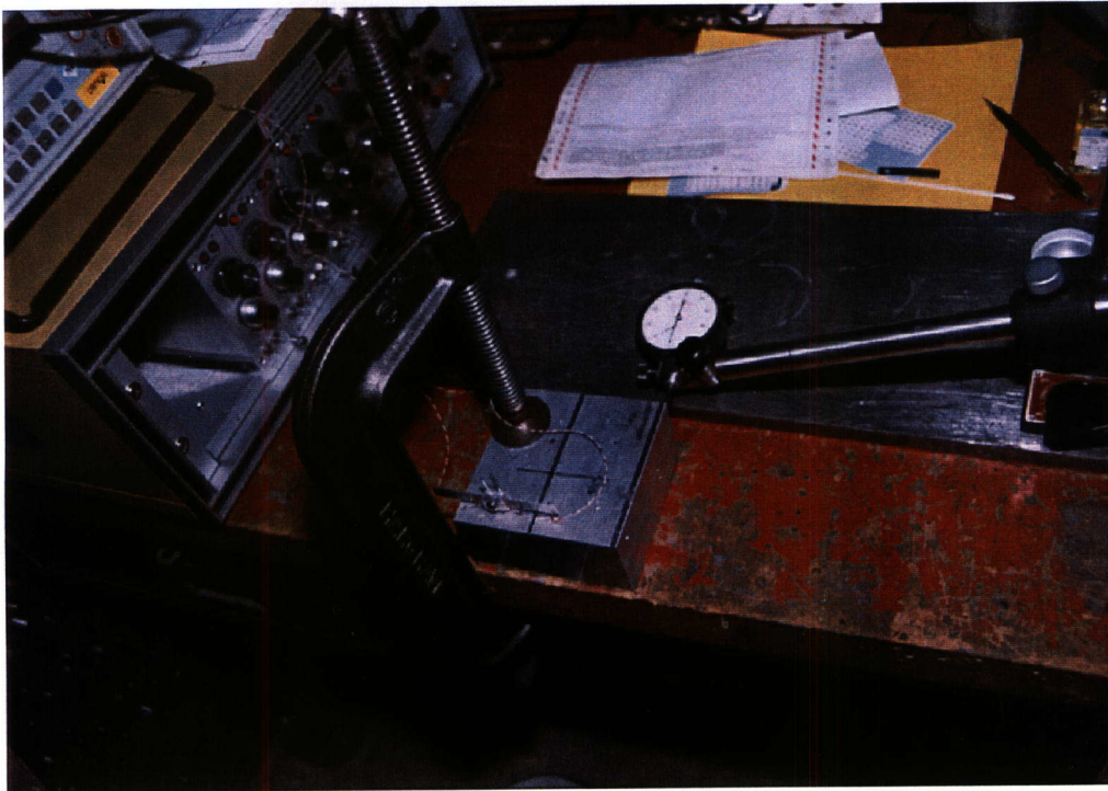
Figure 6-3. Calibration apparatus for cantilever beams
