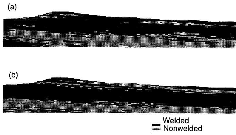
Figure 6-6. Representative west-to-east cross-section of Yucca Mountain illustrating the tendency of simulated welded and nonwelded lithologies to pinch and swell and to interfinger in a more complex fashion than is believed reasonable based on field observations. (a) Profile simulated directly using the anisotropy ratios from Table 6-1. (b) The same profile simulated by adjusting anisotropy ratio 2 to 0.025 (40:1).
