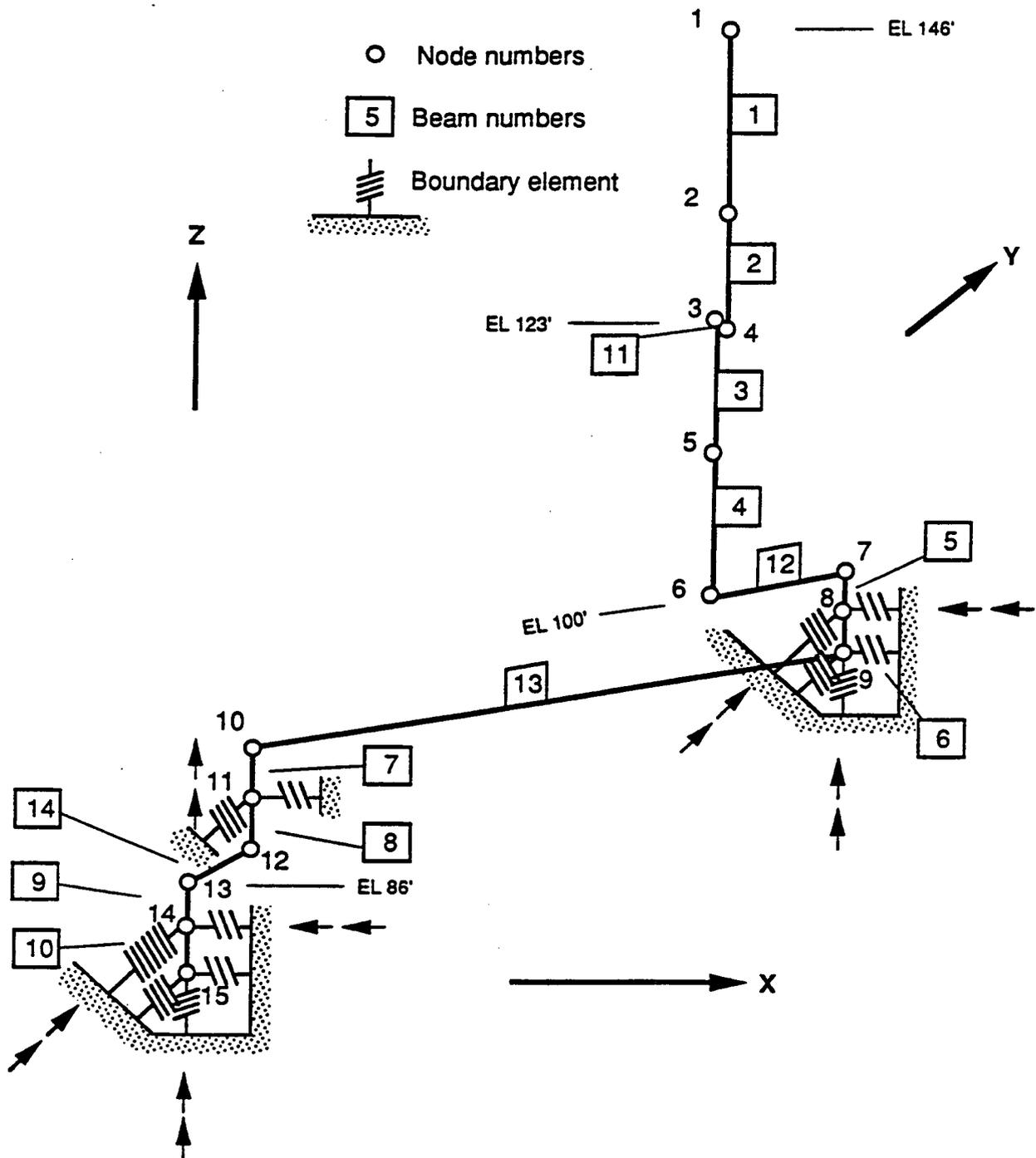
Figure 3-3. VF stick model used by Dames & Moore (Gates, 1993)
