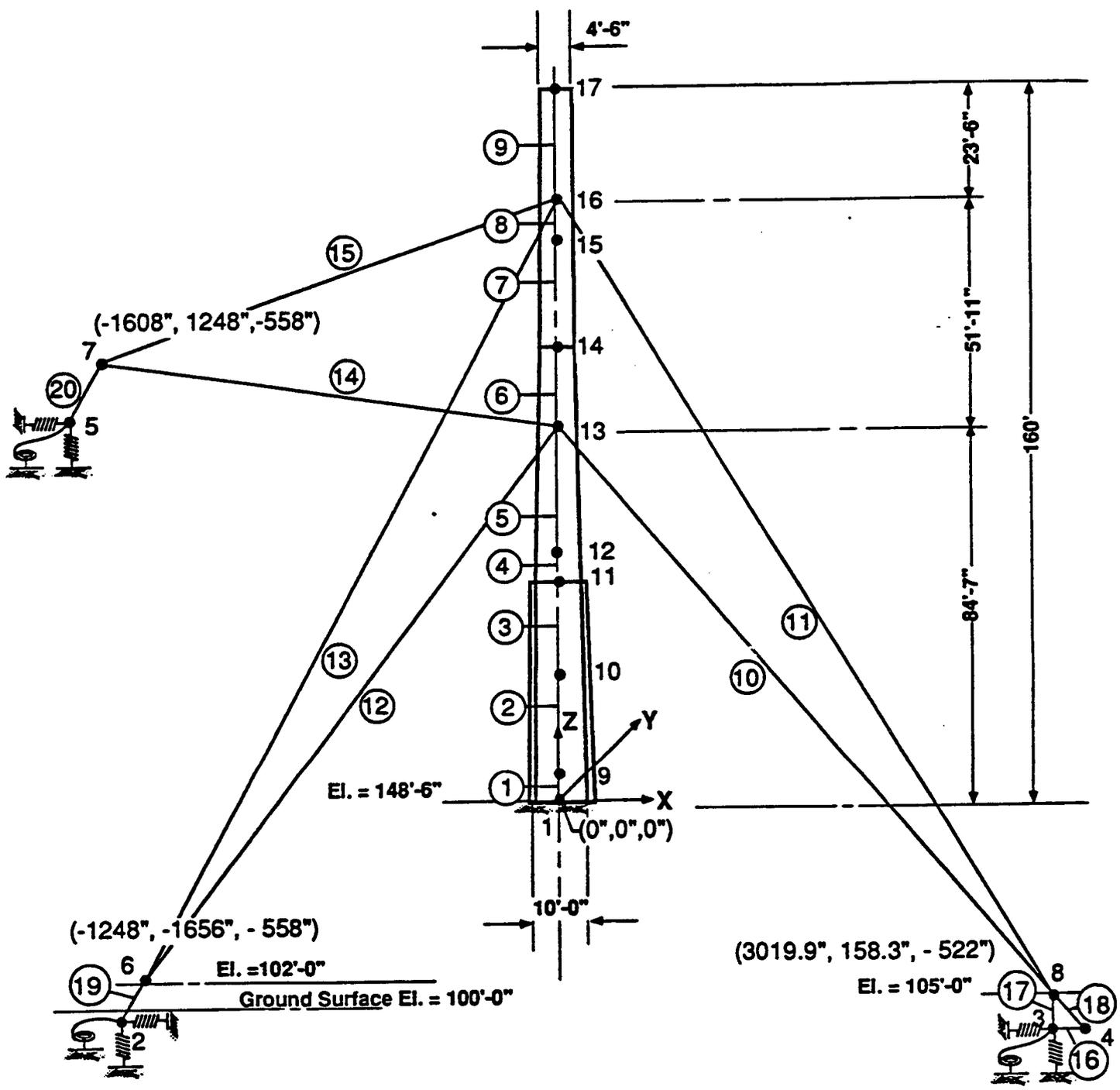
Figure 3-4. Dames & Moore FEA model of reprocessing plant guyed stack (Gates, 1993)
