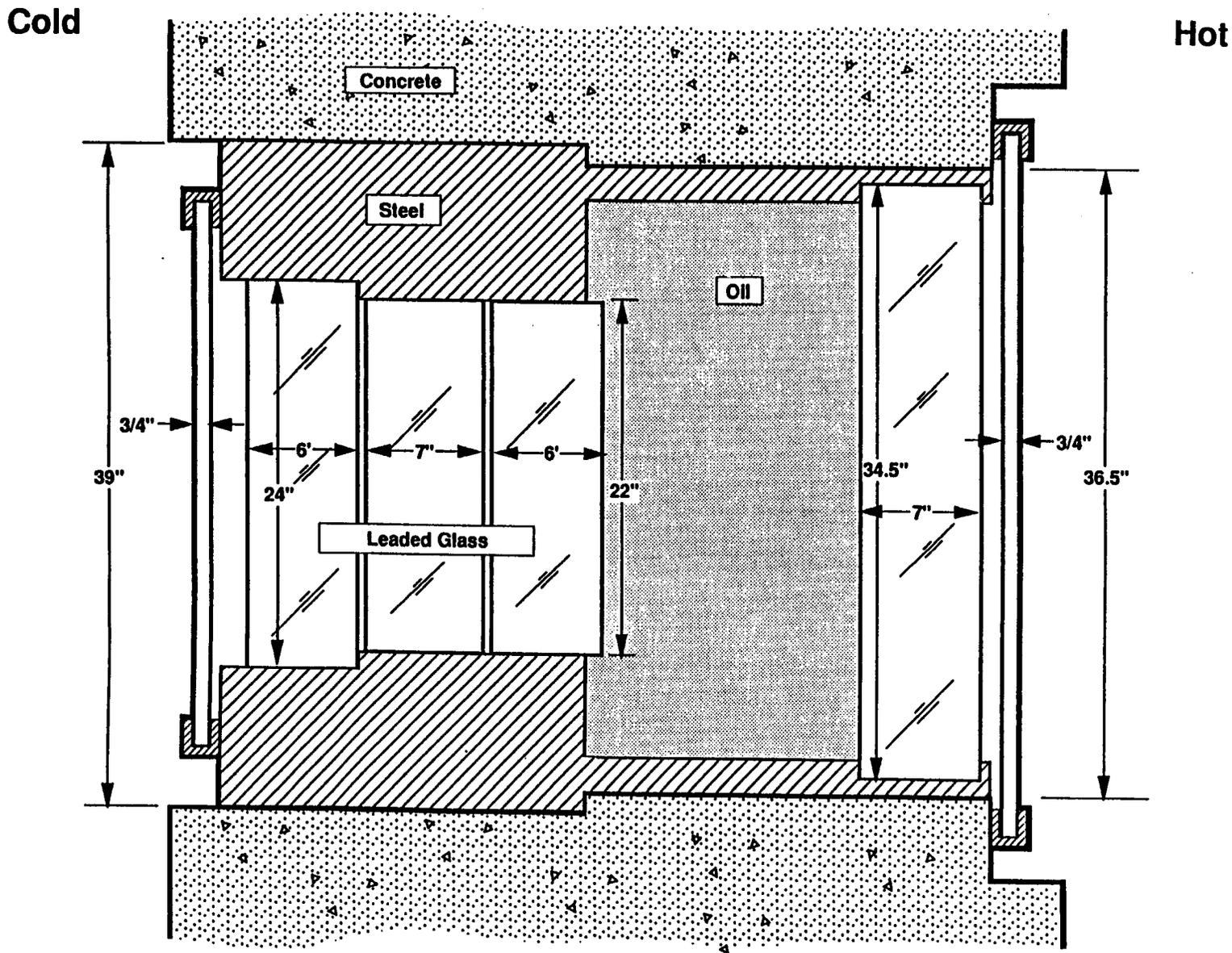
Figure 4-1. Geometry of the shield windows (Gates, 1993)
