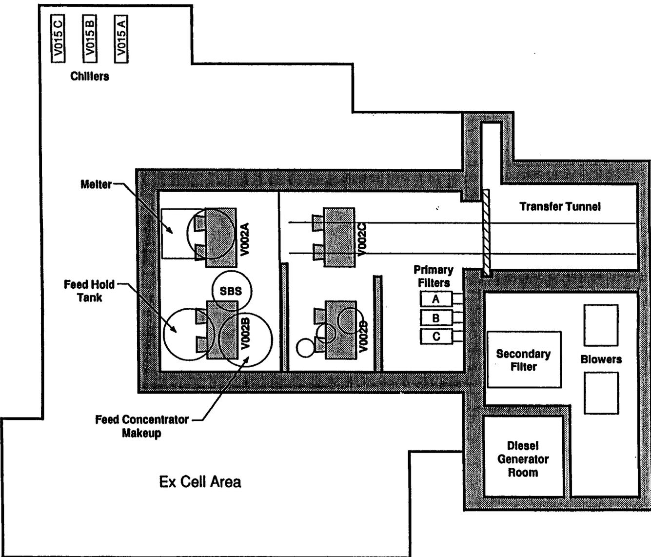
Figure 2-1. Vitrification facility plan (Gates, 1993)
