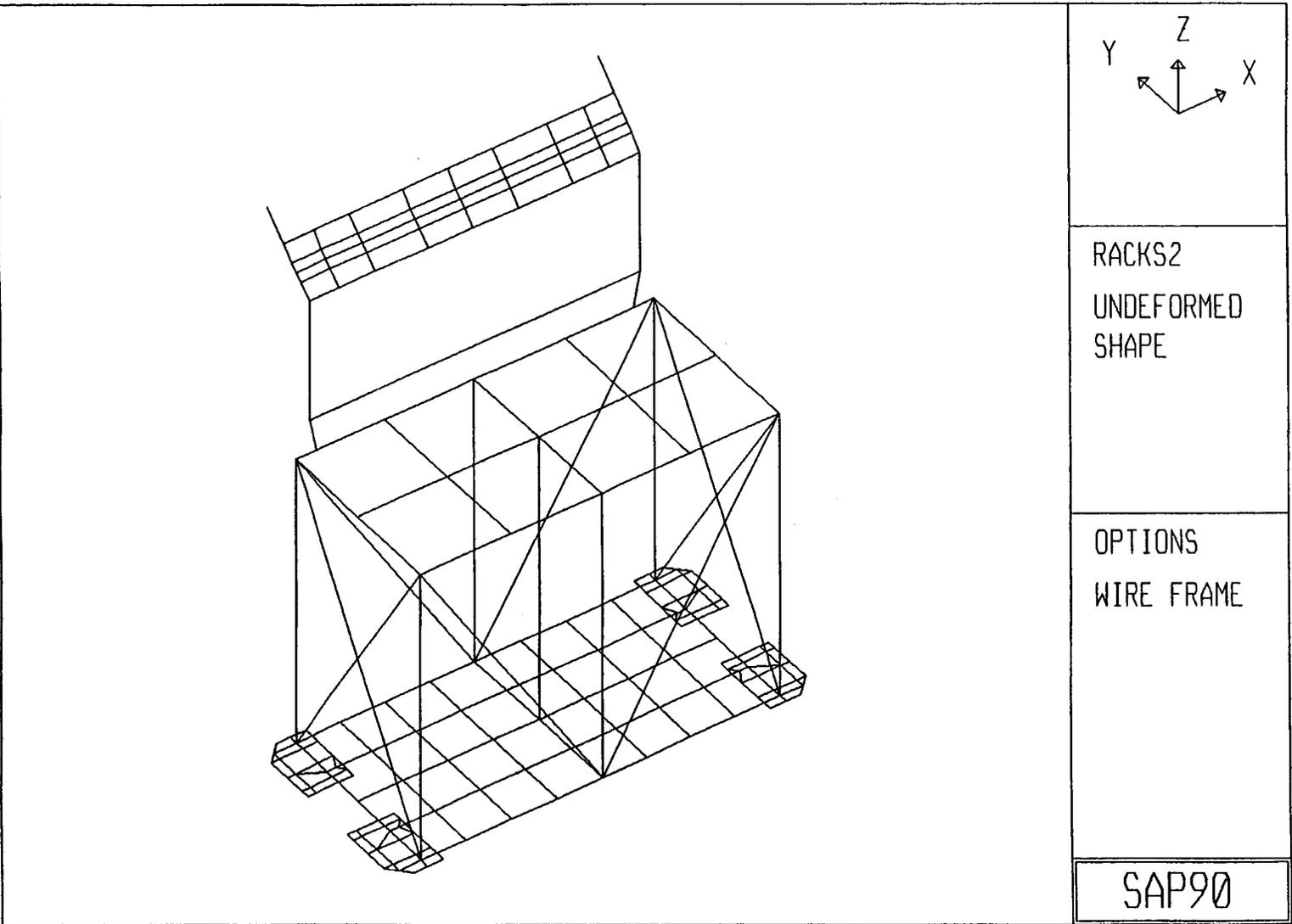
Figure 3-6. FEA of canister storage racks and waste header guide used by Dames & Moore (Gates, 1993)
