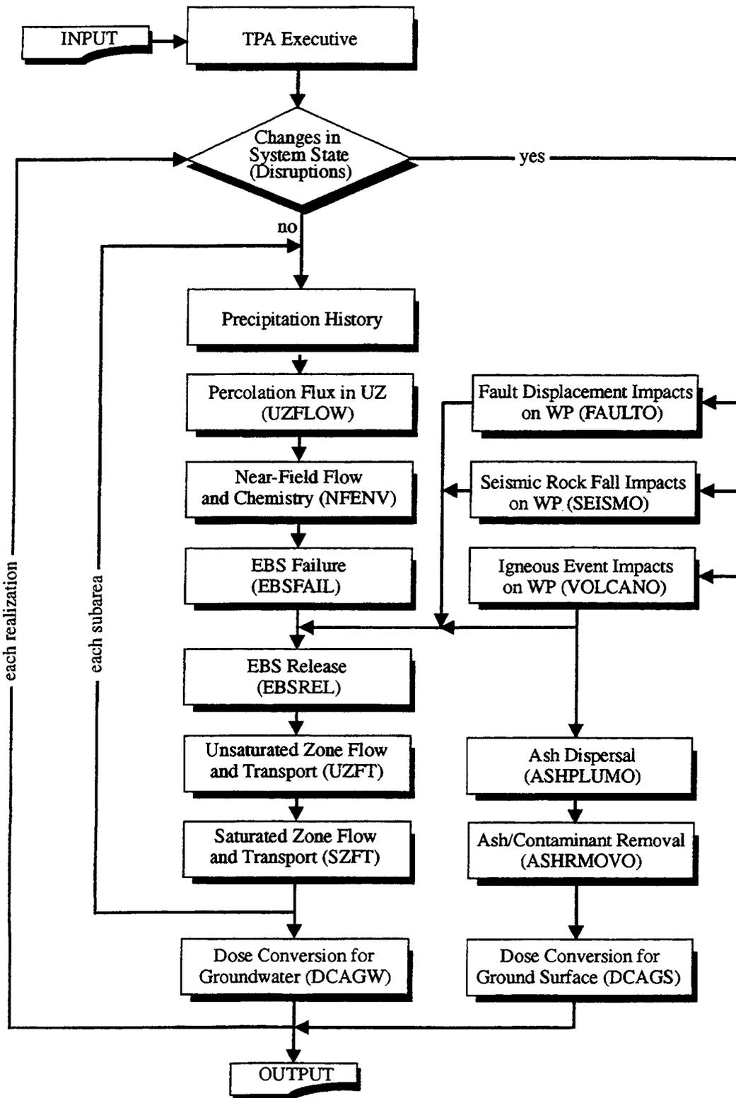
Figure 1-1. Total-system Performance Assessment Code Version 3.1 structure
