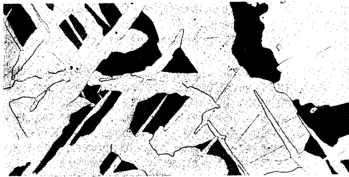
a. Plate NRC-11 Heat-Affected Zone in Region of Crack Growth
