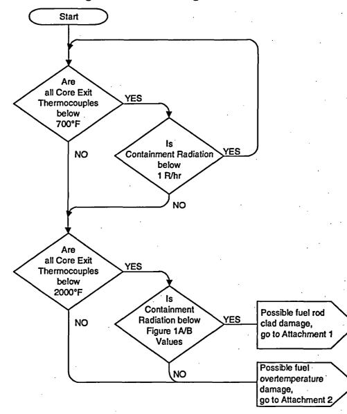
**High Level Core Damage Assessment Flowchart**
