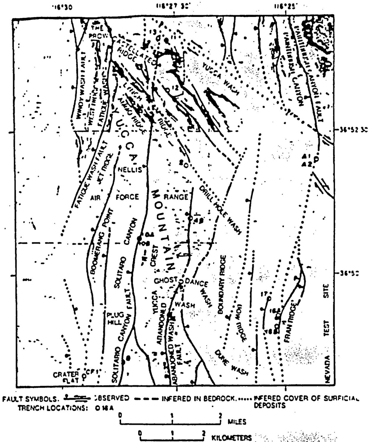
Figure 4. Trenches located along faults at Yucca Mountain interpreted from geologic mapping
