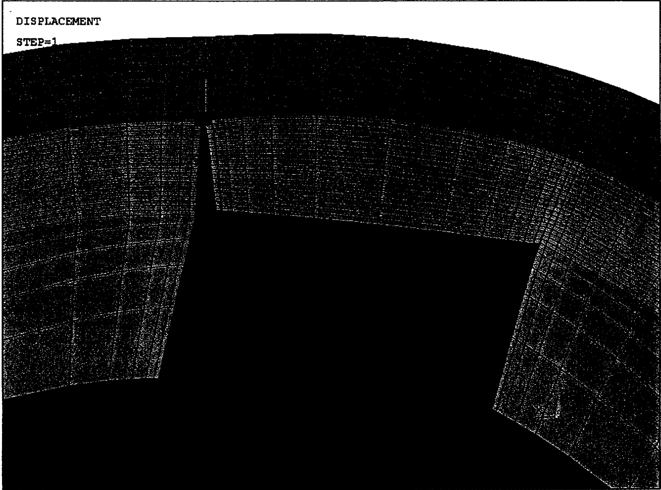
Figure 11: Deformed Shape of the 50% Crack
