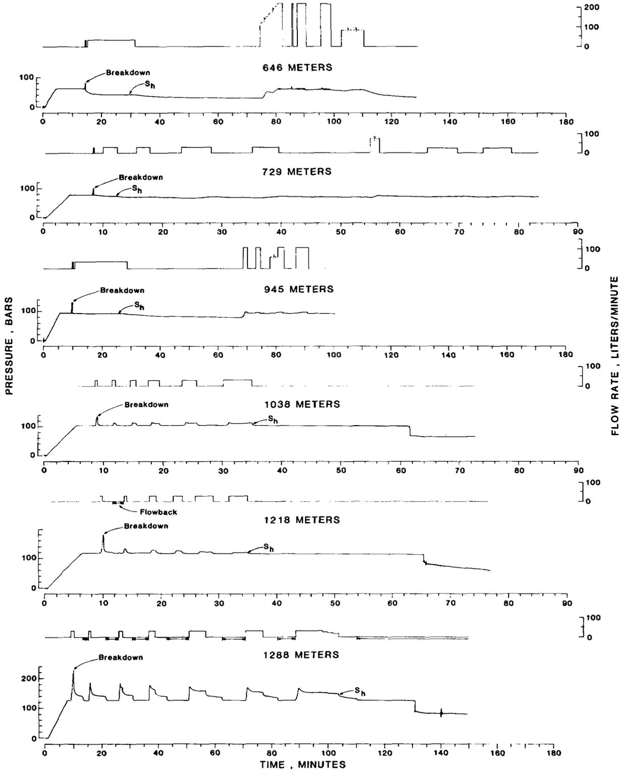
Figure 6. Downhole pressure and flow data for hydraulic fracturing stress measurements in USW-G1. Values chosen for  $S_h$  are indicated.
