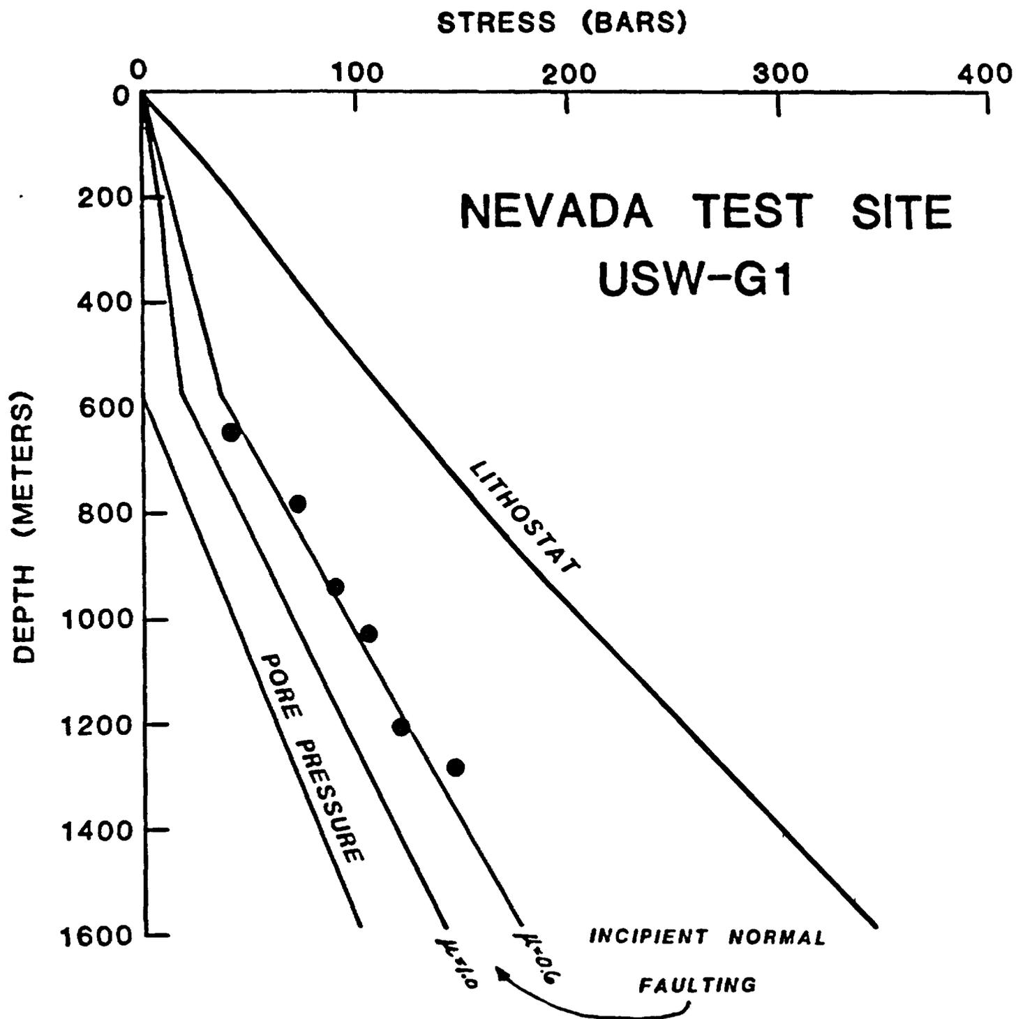
Figure 7. Least principal compressive stress,  $S_h$ , as a function of depth. The vertical stress (lithostat) and pore pressure at depth are shown for reference.
