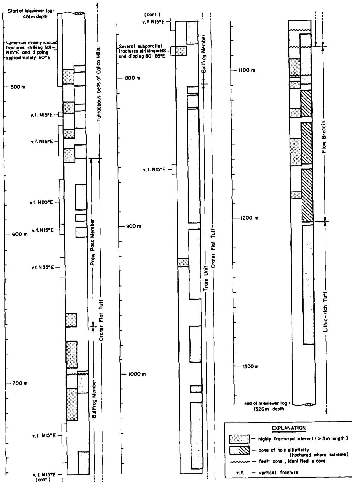
Figure 2. Log showing major features (vertical fractures, highly fractured intervals, and hole ellipticity) observed on televiwer log. Stratigraphy, static water level, and known fault zones identified from core also shown.
