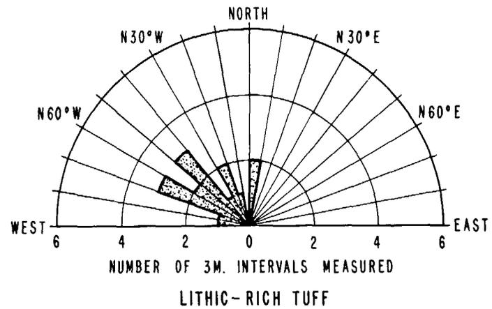
Figure 5. Rose diagram showing orientations of hole ellipticity (long axis) within the a) Calico Hills, Prow Pass, and Bullfrog units, b) Tram unit, c) Flow Breccia, and d) Lithic-rich tuff. Orientations were measured for 3-m-long zones in which ellipticity was well defined and the wall rock was relatively unfractured.
