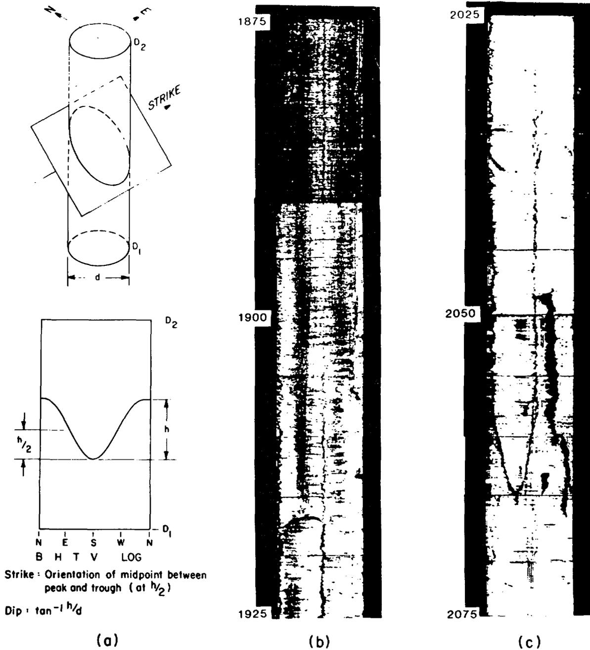
Figure 1. a) Isometric sketch of fracture or bedding plane intersecting borehole and corresponding borehole televiwer log [after Zemanek et al. (1969), fig. 7];
