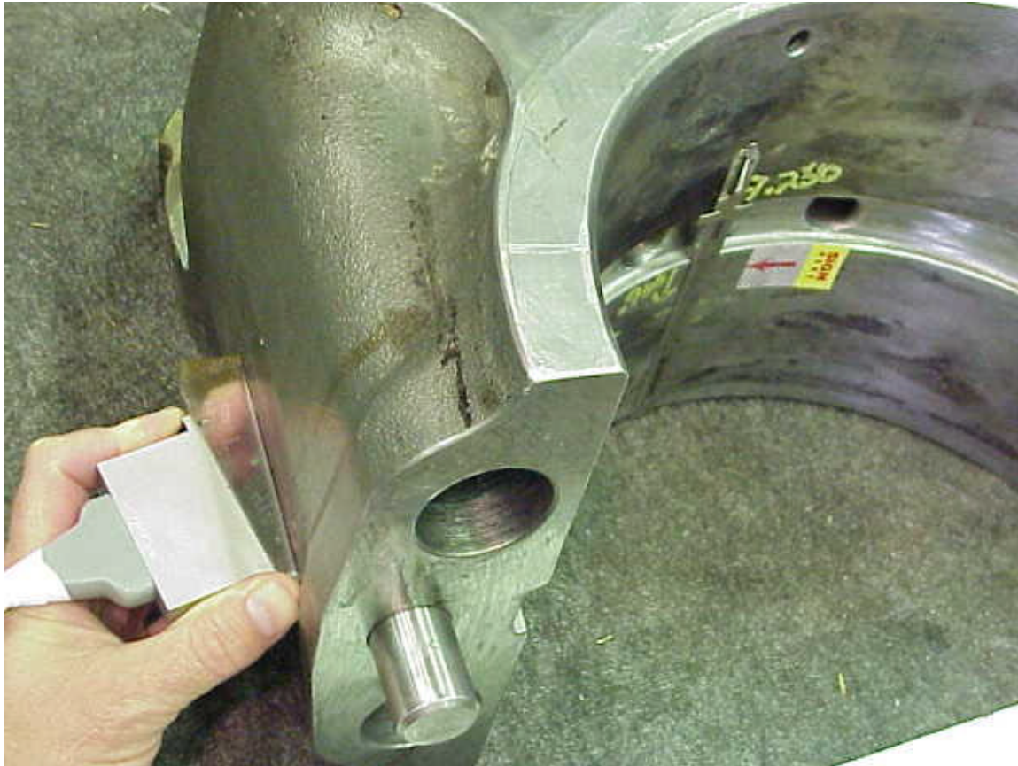
Fig 3. Calibration standard showing scanning surface of transducer
