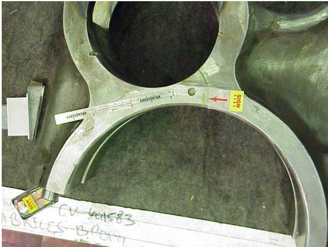
Fig 5. Side-view showing location of EDM notch
