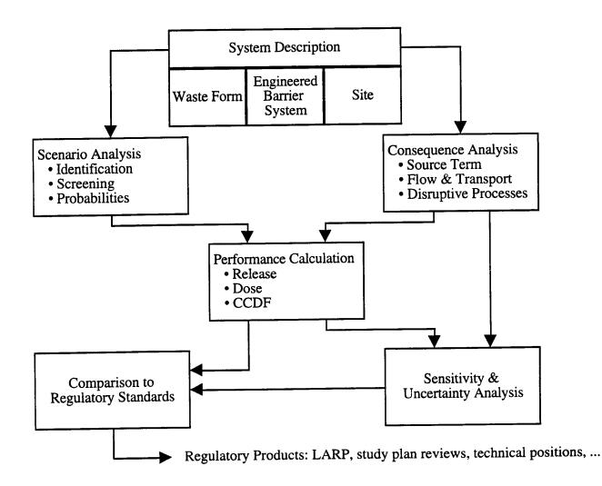
Figure 3-1. Components of a total system performance assessment
