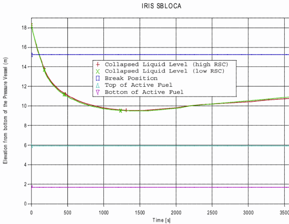
Figure 2.6-12 4" CVCS Line Break – Reactor Coolant System Fluid Mass and Collapsed Liquid Level Transient (Different position of the SG check-valves)
