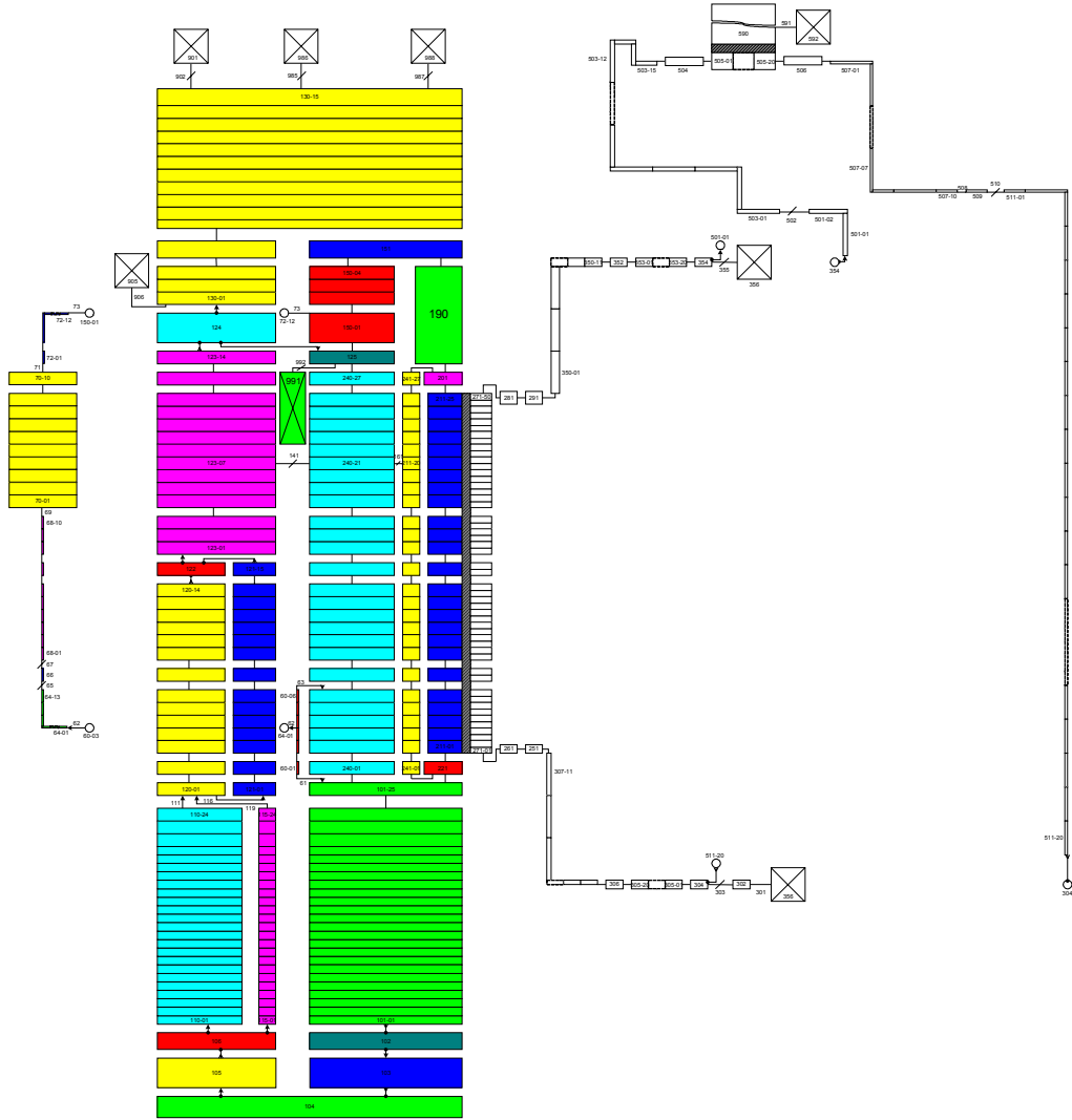
Figure 1. Overview of IRIS nodalization for RELAP5 Mod3.3
